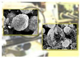
Better processing leads to better batteries. At left, broken particles of oxide in a lithium-iron-phosphate-based electrode show incomplete coating of carbon on their surfaces, which decreases electrode performance. At right, improved mixing of materials generates whole particles, better coated with conductive carbon.
