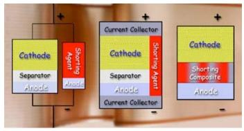
Polymer "shorting agents" can redirect the flow of current when a battery is fully charged. Reversible shorting agents can be used outside the cell (left), as an extra internal component of the cell (middle), or as a composite in the separator between anode and cathode (right).
