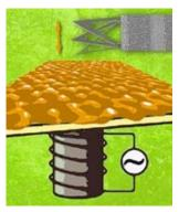
Current-sensing atomic force microscopy is used to measure both the conductance and the surface topography of electrode materials, with resolution at micrometer and nanometer scales.
