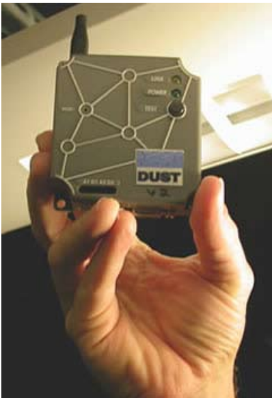
The Dust Networks mote shown here is part of a prototype lighting control system being tested to demonstrate wireless control of office fluorescent lighting for greater energy efficiency and occupant comfort.
