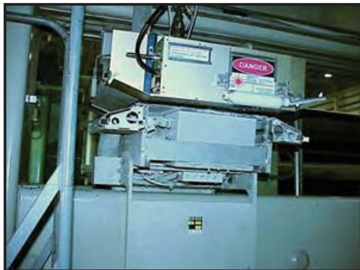
Figure 1. The laser ultrasonic sensor was successfully tested at a working paper mill.
