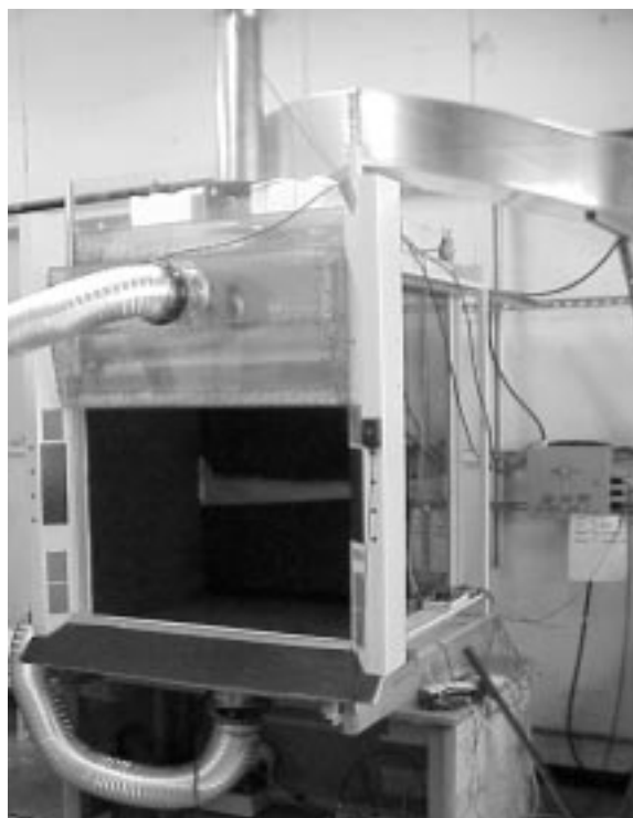
A low-flow fume hood could be part of an energy-saving strategy for high-tech industries.
