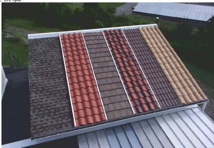
Figure 4. Testing cool-colored roof materials at Oak Ridge National Laboratory on the Envelope Systems Research Apparatus.
