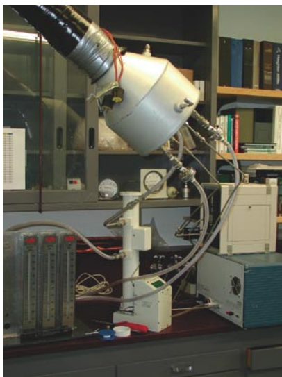
Figure 3. The evolved gas analysis system (Photo courtesy Ted Gartner)
