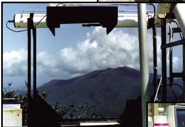
Figure 2. Sampling location at El Yunque Peak, Puerto Rico. The instrument measures the light reflected from cloud drops.
