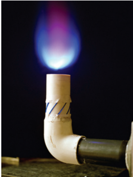
Figure 1. Laboratory UCLSB prototype with 5 cm internal diameter, firing at a rate of 15 kilowatts. This burner is made entirely out of plastic components to showcase its unique lifted flame feature.
