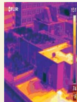
"Green roofs" are cooler than the surrounding conventional roofs.
