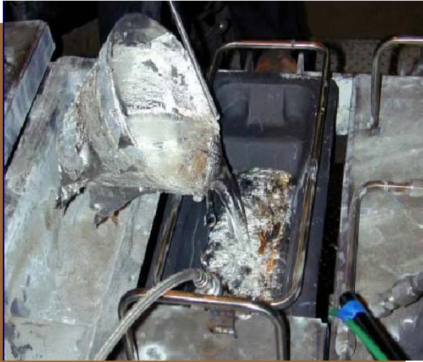
Figure 1. Molten Mg with SF 6 cover gas.
