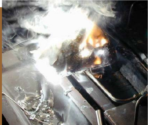
Figure 2. Molten Mg without protective cover gas.
