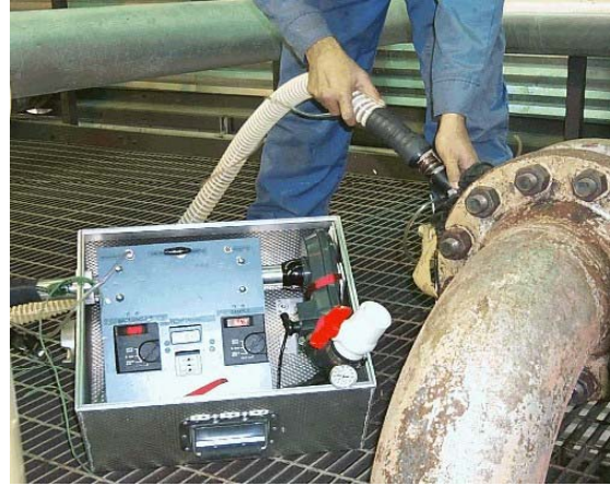
Hi-Flow™ Sampler to measure emission rates.
