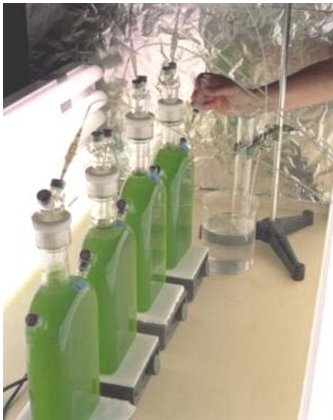
A photoconversion process to produce hydrogen from metabolically engineered algae.
