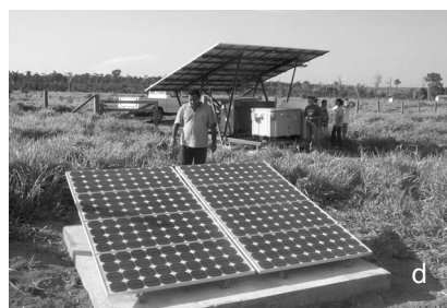
In situ field measurements in the Santarem region: a) measuring wind direction and speed, air temperature and precipitation, b) field laboratory, c) CO 2 flux and profiles, d) solar panels provide energy for continuous field measurements, e) tower flux measurements above the canopy of the Tapajos National Forest.
