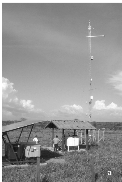
In situ field measurements in the Santarem region: a) measuring wind direction and speed, air temperature and precipitation, b) field laboratory, c) CO 2 flux and profiles, d) solar panels provide energy for continuous field measurements, e) tower flux measurements above the canopy of the Tapajos National Forest.
