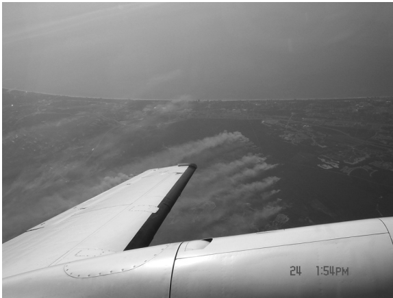
Langley researchers Mike Wusk, Ray Rogers, and pilot Les Kagey flew a King Air B200 equipped with a High Spectral Resolution Lidar over the wildfires in South Carolina to measure the behavior of the smoke plume produced by a blaze that ultimately burned 19,600 acres of land. To view photo in color please visit: www.nasa.gov/topics/earth/features/myrtlebeachfires.html . Credit: Mike Wusk/NASA HSRL Team.
