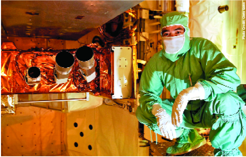
Goddard engineer Bo Naasz successfully demonstrated the Relative Navigation System (RNS) during the Hubble Servicing Mission. He is pictured here with RNS, which was installed inside the Shuttle cargo bay.
