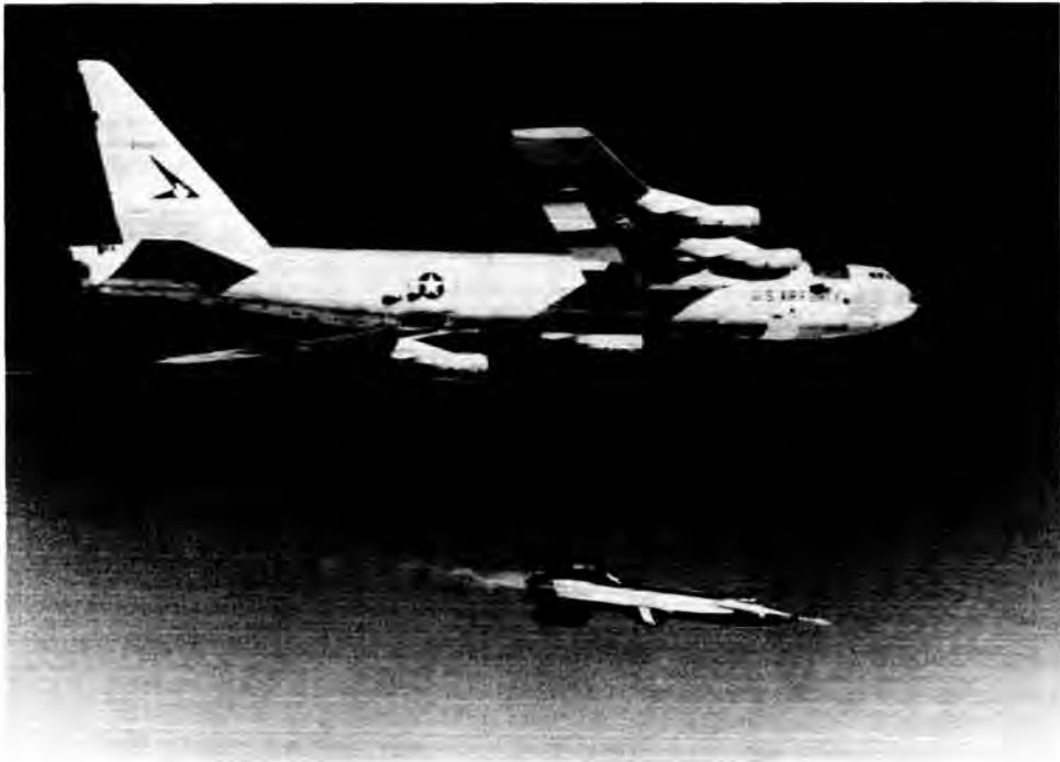
Fig. 4. The number one X-15 just after being launched on June 8, 1959. This is Scott Crossfield's first glide flight flown with the X-15 nose boom, North American Aviation livery, and the XLR-11 engines. (E88-013-15).
