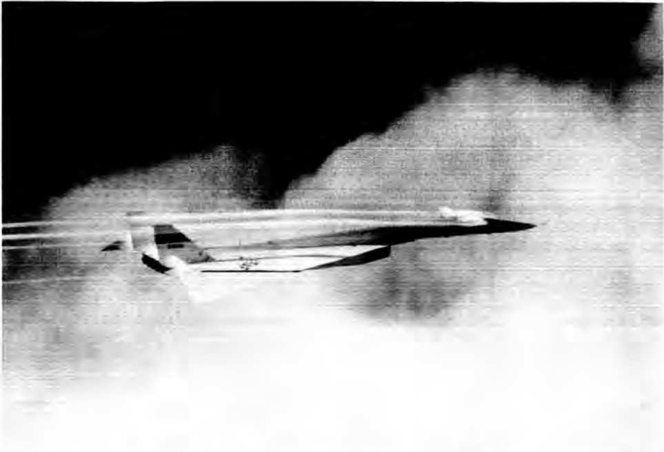
Fig. 3. August 10, 1967 flight of the XB-70A number one during a test to intentionally demonstrate the complex vortex flows generated by the vehicle as it experienced natural condensation in the humid atmosphere. (E-17462)
