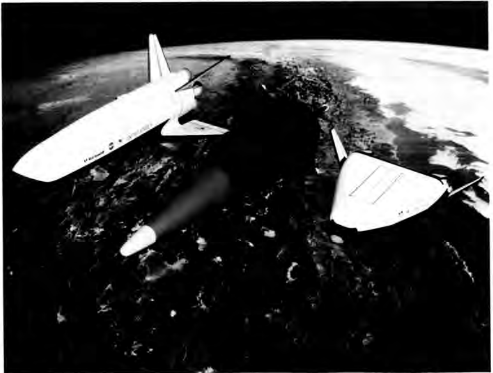
Fig. 1. Three industry proposed SSTO vehicles on which they based their X-33 designs. From left to right: The Rockwell wing-body vehicle, the McDonnell-Douglas vertical lander, and the Lockheed lifting body. (EC95 43320-1)
