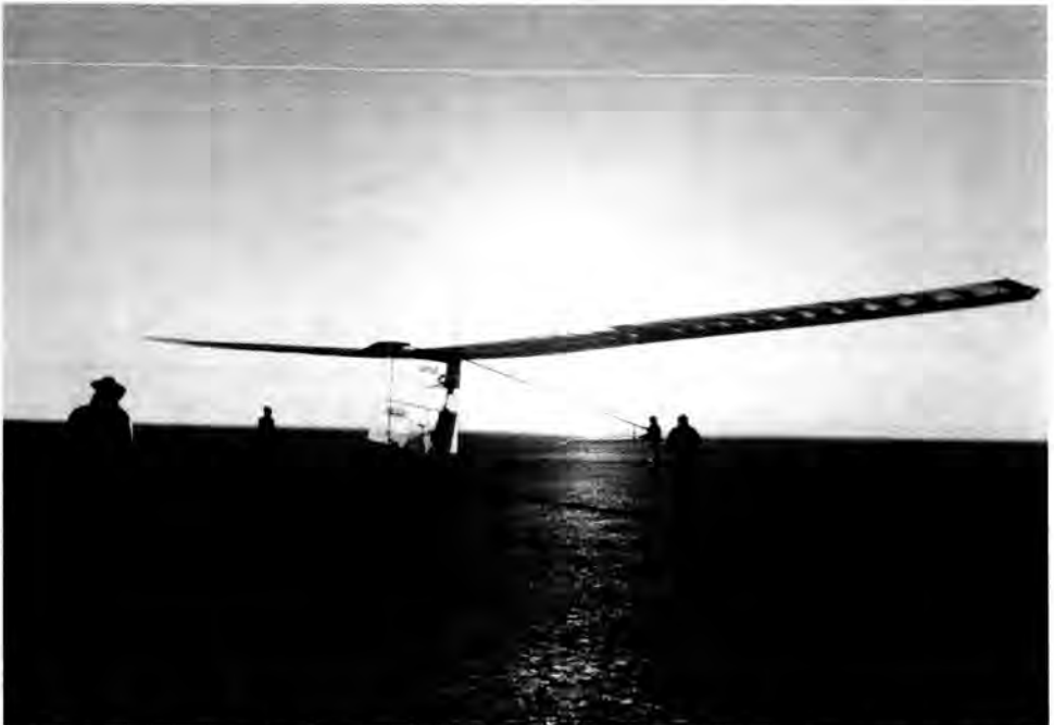
Fig. 3. The Gossamer Albatross preparing for a sunrise flight at Dryden in April 1980. Shortly after the manpowered Albatross successfully flew across the English Channel, it was brought to Dryden for an instrumented flight test program to evaluate its lift, drag, stability and control, and thrust characteristics. (ECN-14339)
