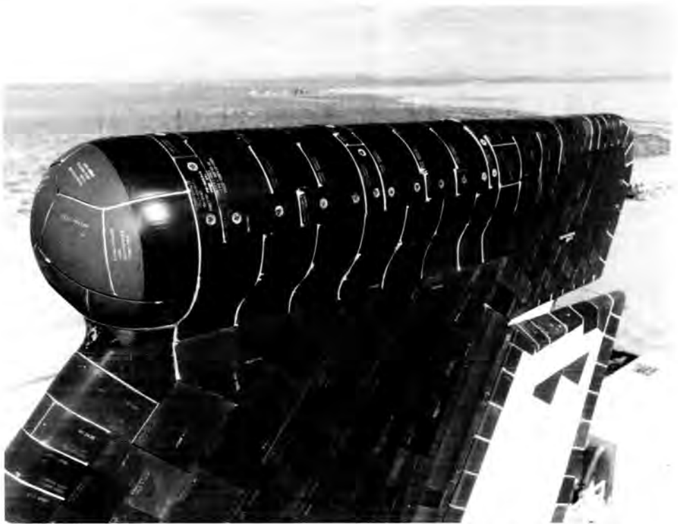
Fig. 7. The SILTS pod on top of the tail of Space Shuttle Columbia. (EC86 33311-33)
