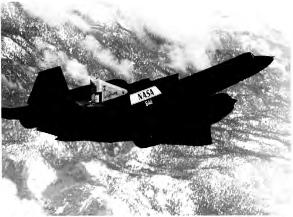
Fig. 2. The SR-71 carrying the LASRE experiment to investigate the in-flight characteristics of the aerospike engine. (EC98 44509-15)
