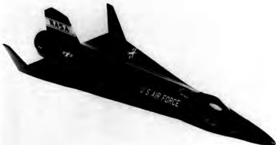
Fig. 2. One of many proposed follow-on X-15 designs with a delta wing modification. (E-13857)
