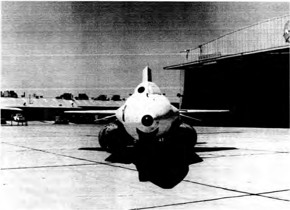
Fig. 2. X-15A-2 in August 1967 prior to the first flight, equipped with the full ablative coating, eyelid, 20-degree dummy ramjet, and external tanks. (E 17339)
