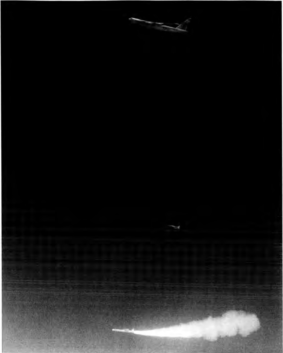
Fig. 2. An early B-52-launched Pegasus shown shortly after rocket ignition, along with an F-18 chase plane. (EC91 348-4)
