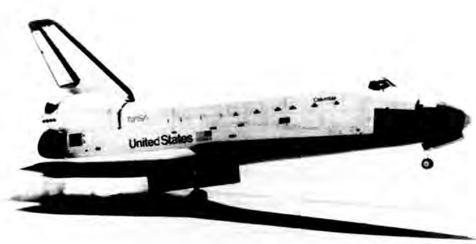
Fig. 1. The Space Shuttle Columbia touching down after orbiting the Earth on STS-1. (EC81 15104)
