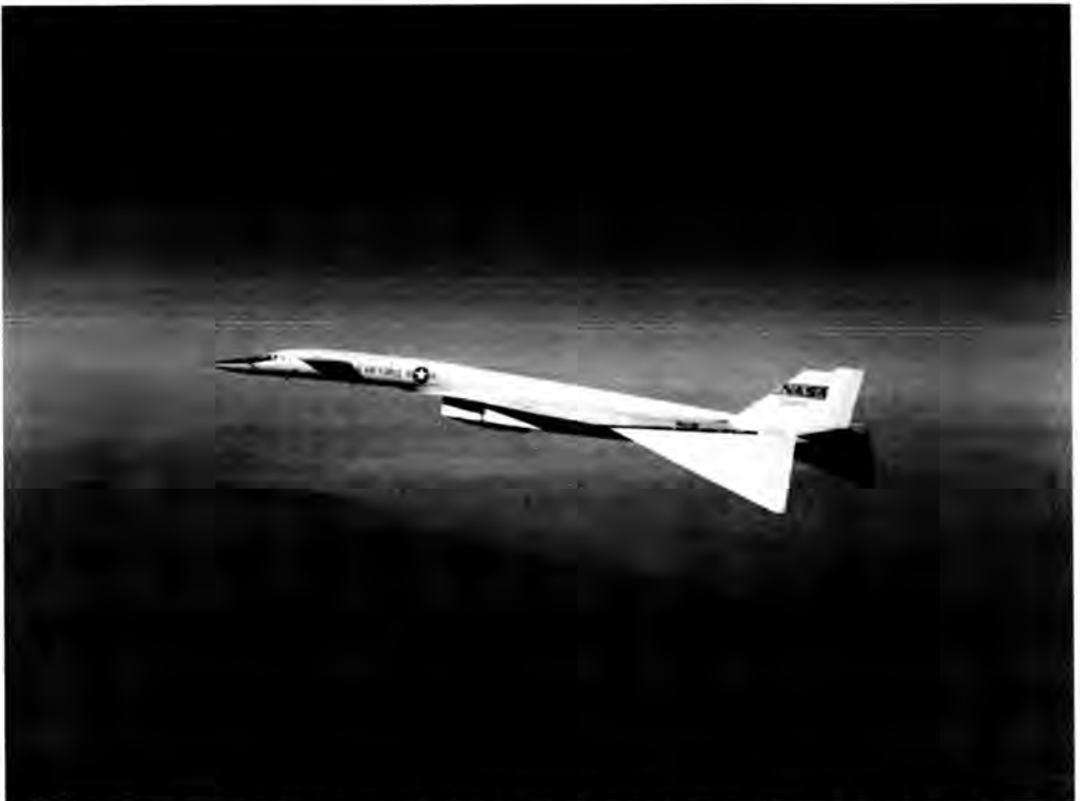
Fig. 7. XB-70A number one with the wingtips deflected on its August 16, 1968 flight. (ECN 2125)
