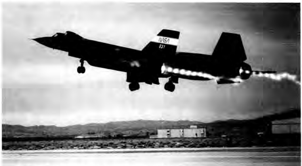
Fig. 4. SR-71B shortly after takeoff showing the shock diamonds in the “twisted” exhaust plumes entrained in the strong aerodynamic vortex shed from the aircraft. (EC92 1284-01)
