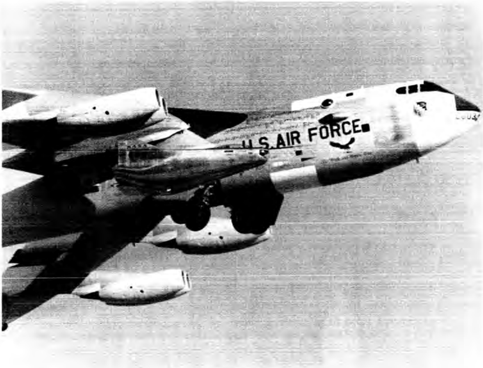
Fig. 2. The M2-F2 mated to the B-52 mothership on climb to altitude on Milt Thompson's last flight on September 2, 1966. (ECN 1437)
