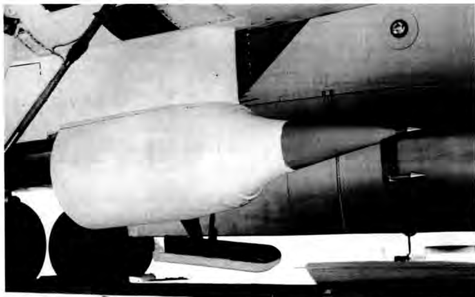
Fig. 3. Dummy ramjet outfitted with the 20-degree cone and the local flow experiment on the 90-degree X-15A-2 ventral fin prior to the August 21, 1967 flight. (E67-17493)
