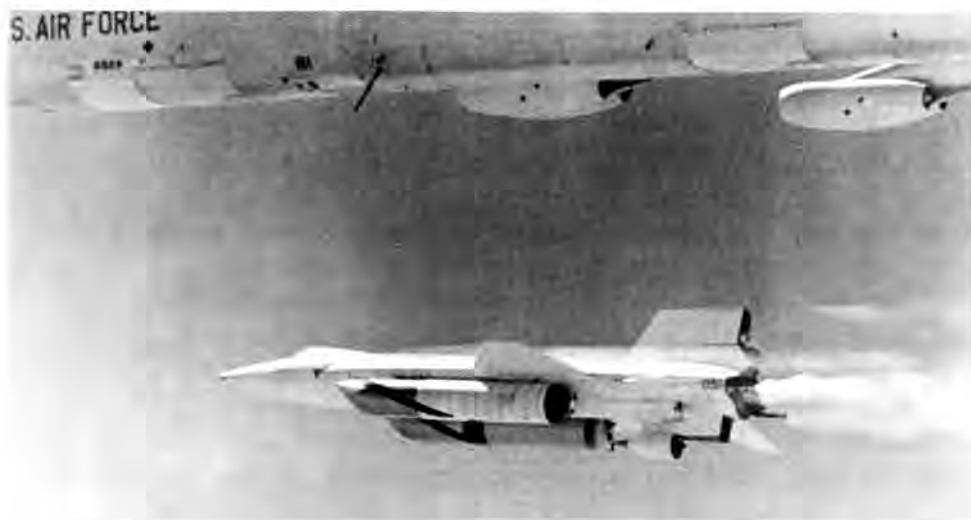
Fig. 4. X-15A-2 with the tanks and full ablative coating a few minutes before reaching its record setting Mach 6.7 speed on October 3, 1967. Pete Knight's flight resulted in shock impingement damage and the loss of the dummy ramjet experiment. (EC68-1889)
