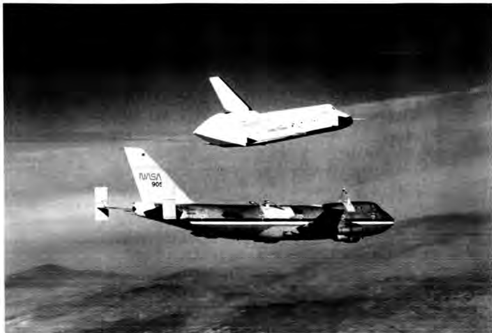
Fig. 1. The first separation of the Enterprise from the SCA with the tailcone on. (E77 8608)
