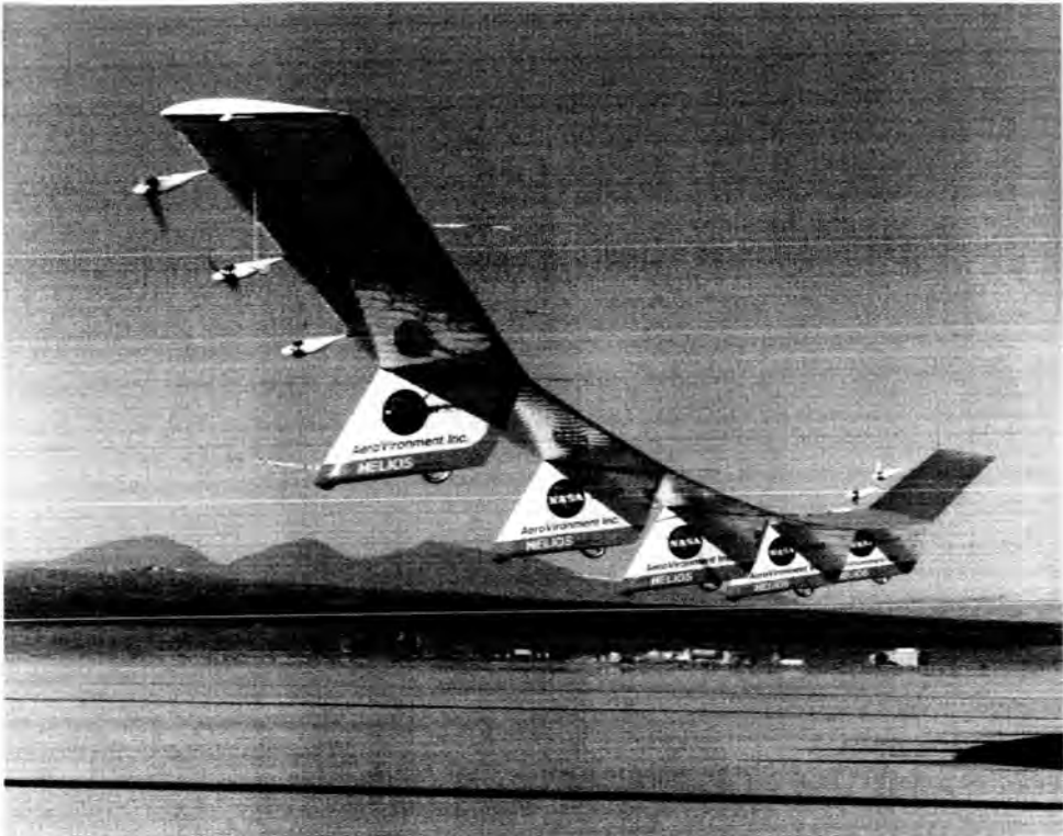
Fig. 4. Helios vehicle being flight tested at Dryden in preparation for its record setting altitude flight in Hawaii. (EC99 45285-5)
