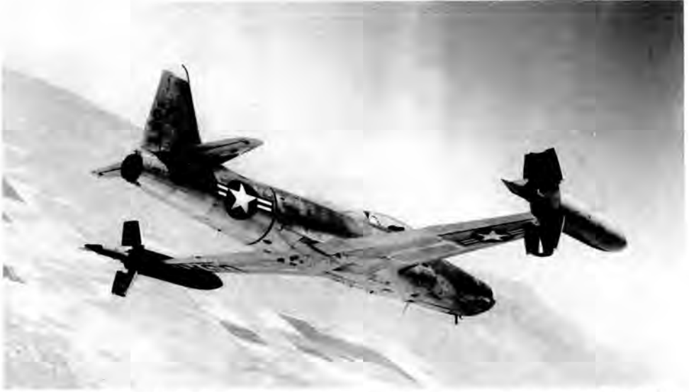
Fig. 3. The Cornell T-33 variable stability aircraft with the drag petals extended. Fred Haise piloted the T-33 to test the M2-F2's stability and control, lift and drag during this April 1965 flight. (E 13020)
