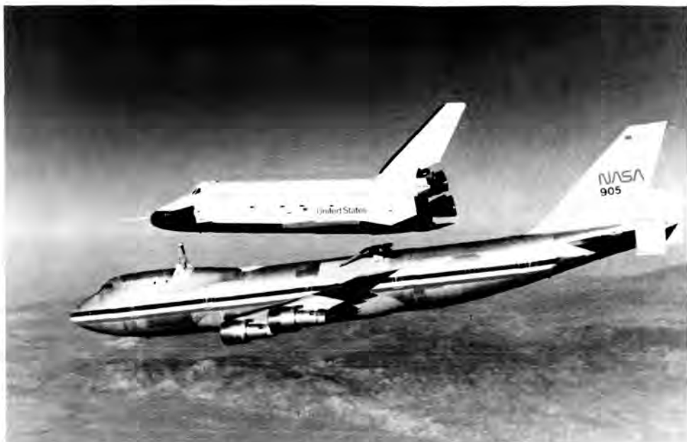
Fig. 2. The Enterprise without the tailcone, separating from the SCA. (E77 8923)
