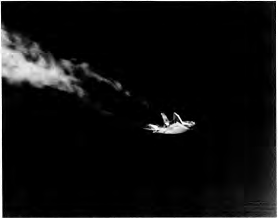
Fig. 9. HL-10 under power with shock diamonds evident during Bill Dana's Mach 1.59 flight of November 17, 1969. (EC69 2347)
