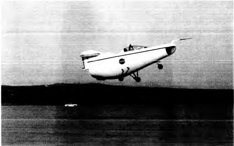
Fig. 2. A photo of the M2-F1 taken immediately after the first release from a car tow, capturing the moment of the very first free flight of a lifting body. Milt Thompson flew the M2-F1 on April 23, 1963. (E 9829)
