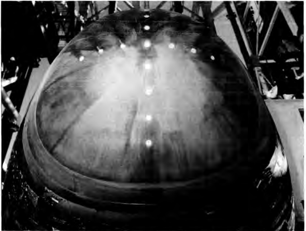
Fig. 6. The SEADS ports are placed in a cruciform configuration on the Space Shuttle Columbia nose as shown in this photo taken after STS-24. (EC86 33311-28)
