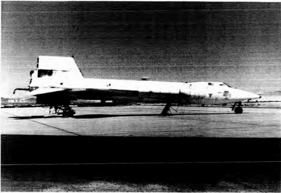
Fig. 5. X-15A-2 after the October 3, 1967 flight showing the scorching of the ablative coating and the absence of the dummy ramjet experiment. (ECN 1834)
