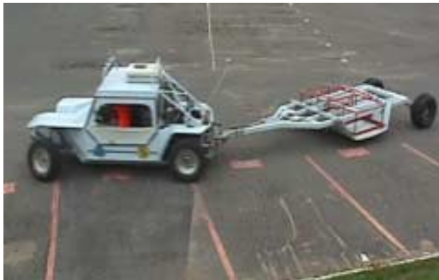
Figure G-1. MTAD's tow vehicle and pulse-induction array deployed.
