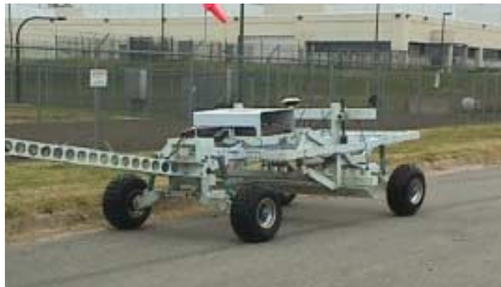
Figure G-3. The MTADS magnetometer array.
