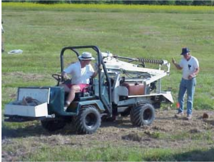
Figure N-4. Positioning the drill rig.
