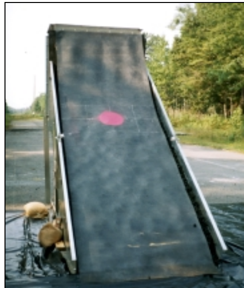
Figure 2-5. Granular rubber friction trap.
