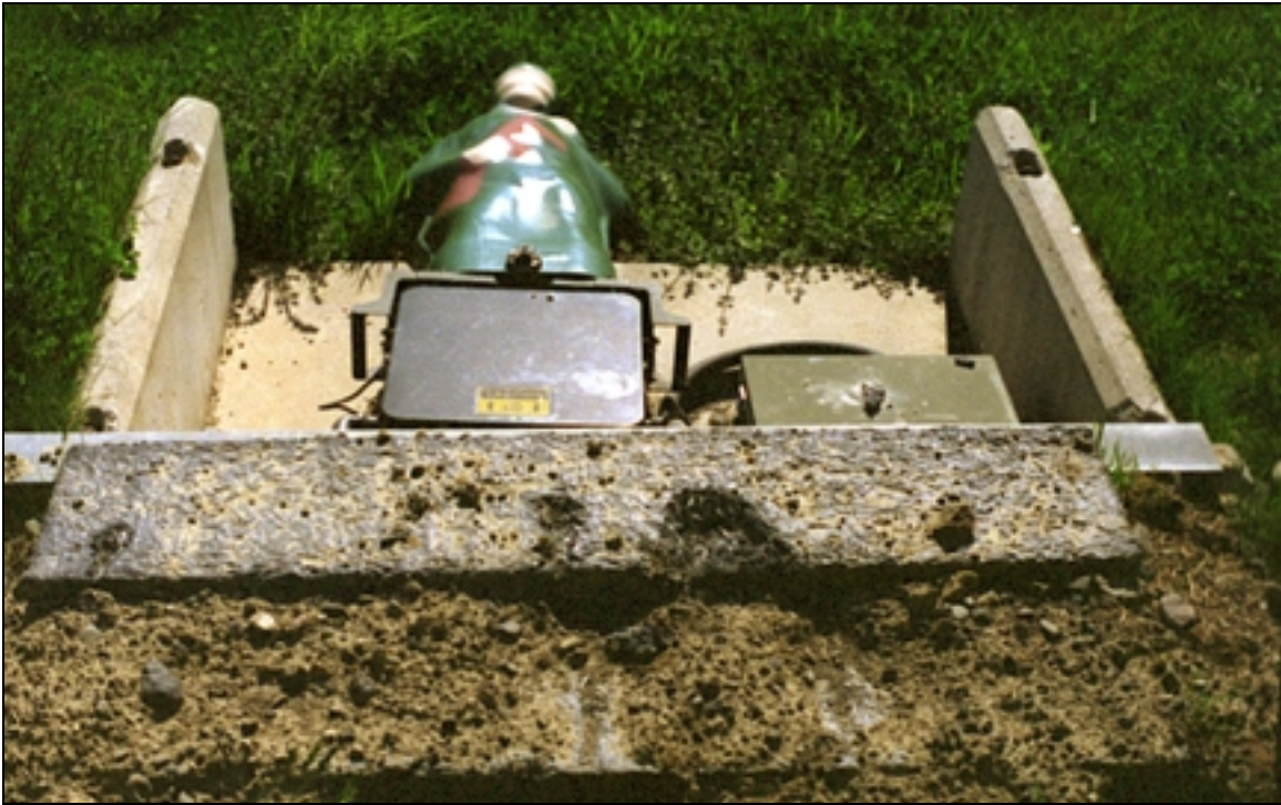
Figure 4-13. SACON blocks protecting target coffin.
