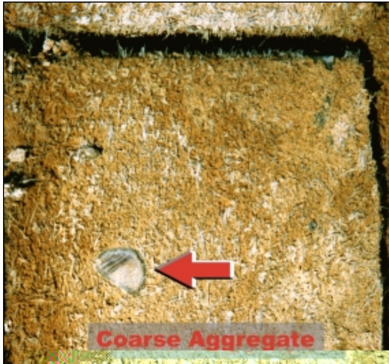
Figure 4-3. Coarse aggregate in 70-lb/ft 3 SACON block.
