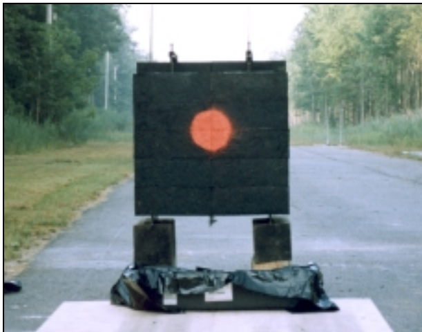
Figure 2-4. Rubber block friction trap.
