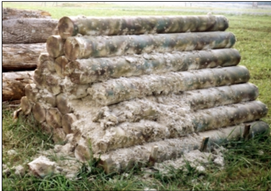
Figure 4-20. SACON simulated log backstop after firing, Morgan Range.
