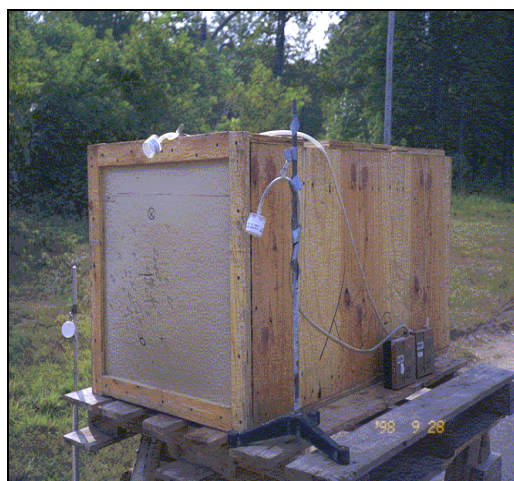
Figure 5-45. Granular rubber test fixture.
