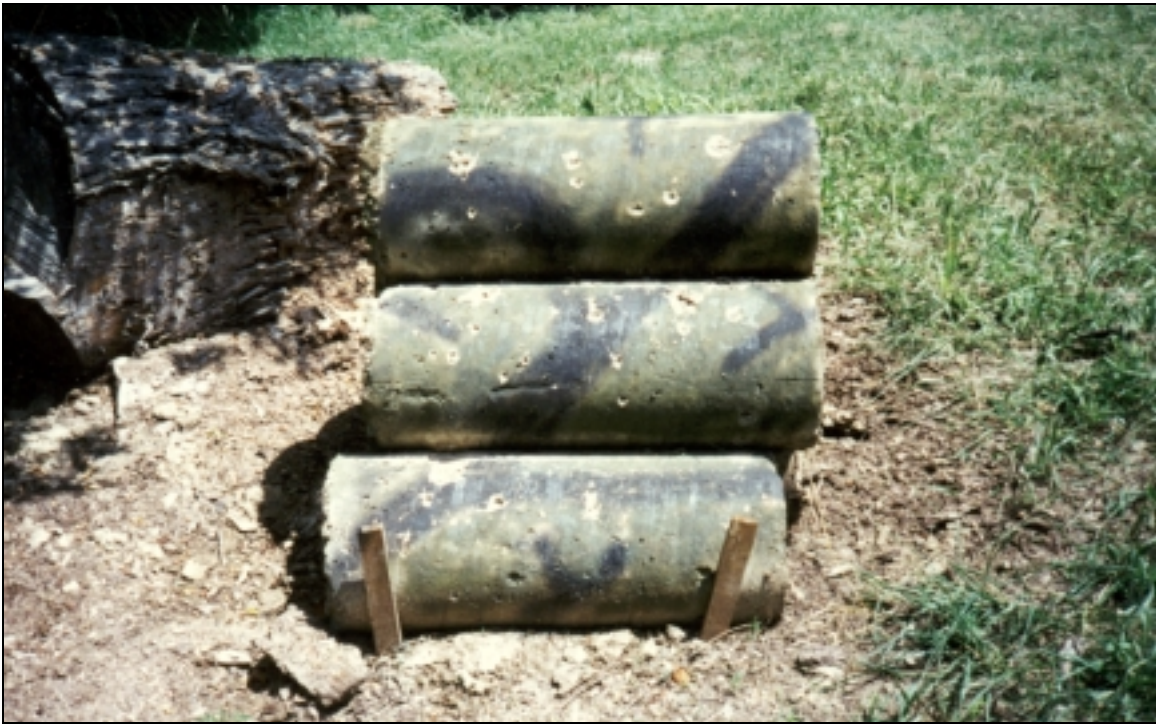
Figure 4-18. SACON "log pile" backstop (Ditto Range, 200-meter target, 26 June 1997).
