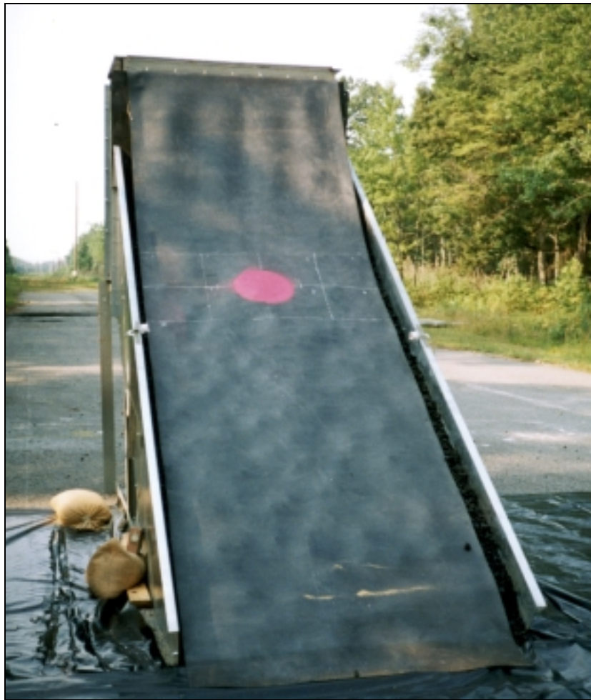
Figure 5-42. Granular rubber friction trap.
