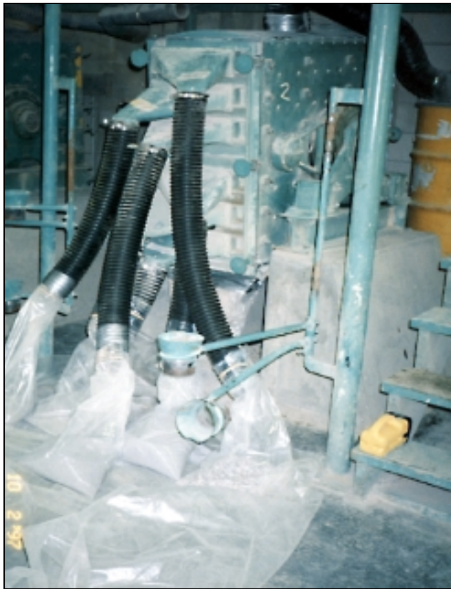
Figure 4-37. Separating sieve fractions.
