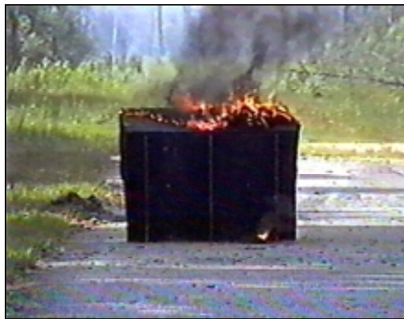
Figure 5-49. Rubber block trap fire (trap tipped on side).
