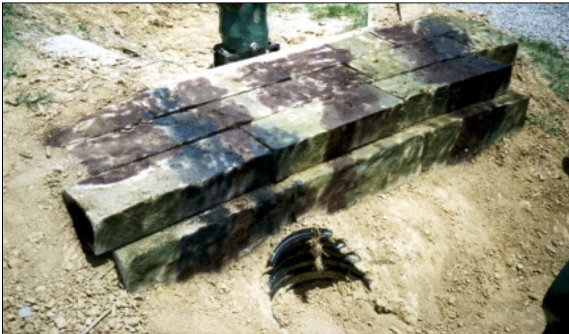
Figure 4-22. Camouflaged SACON railroad ties protecting target coffin.
