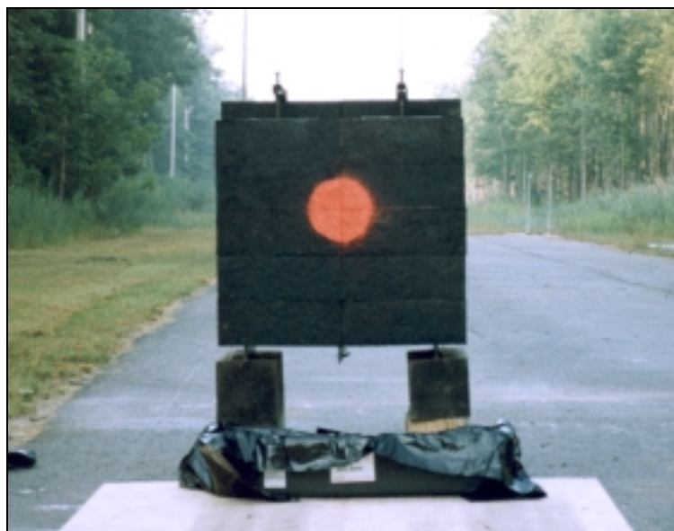
Figure 5-46. Rubber block friction trap.
