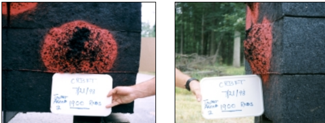
Figure 5-47. Accelerated durability after 1900 rounds (front and side views).
