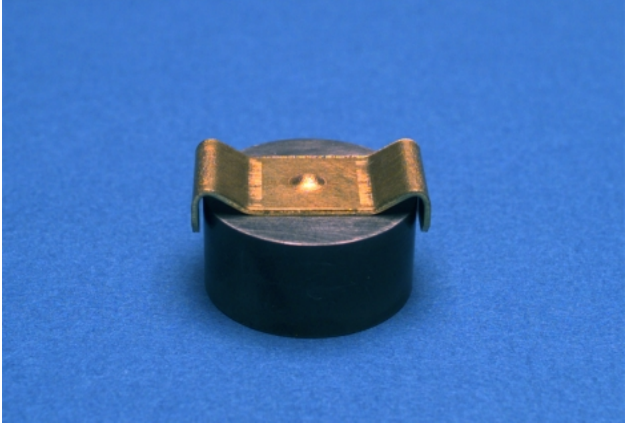
Figure 1. Bimetal Couple Corrosion Test Specimen Pair.
