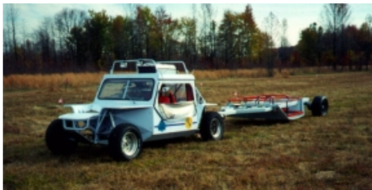
Figure 2 - The EM-61 system in operation.
