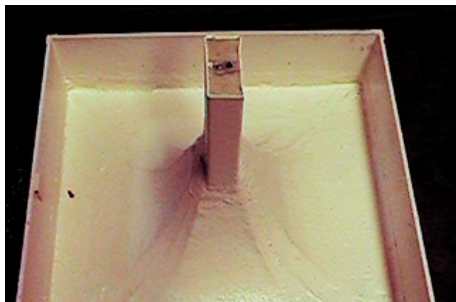
Figure 1 The New ESL Dual-Polarization GPR Antenna Filled with Low Loss Dielectric Material
