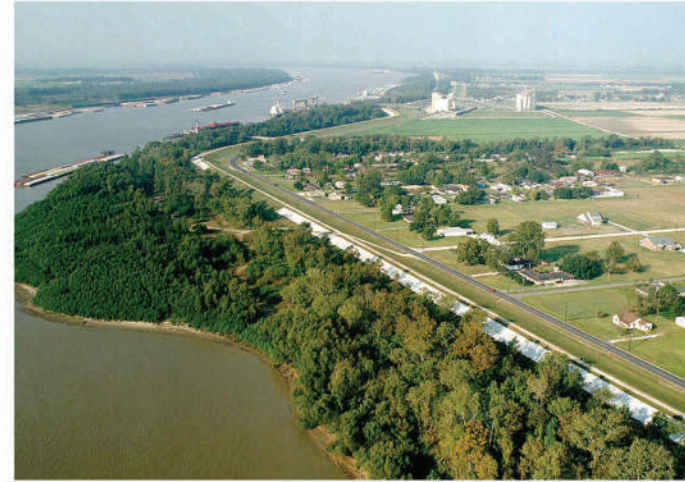
Levees, built by land owners as early as 1717, are constructed for flood control and to aid navigation.
