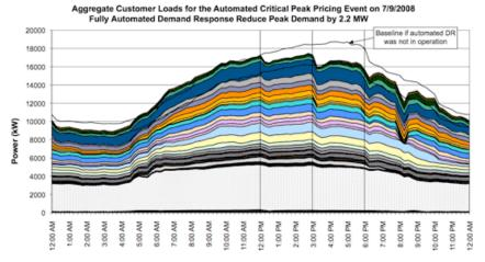
Tests of automated demand response in commercial buildings throughout California show significant reductions in peak electricity load. The white area under the baseline curve represents the amount of power not used because of automated demand response. These tests are being conducted as part of a multi-year testing program funded by the California Energy Commission's Public Interest Energy Research program. This graph includes data from 28 sites around California.
