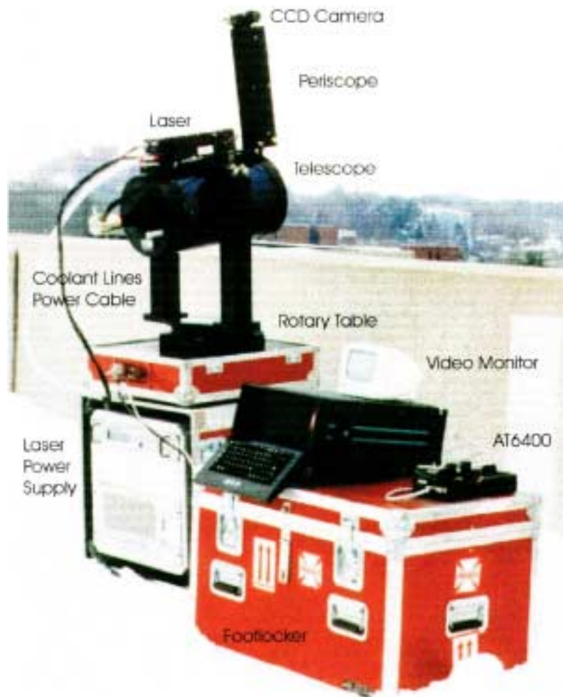
Fig. 1 The LIDAR set up in a typical data collection mode. The major components are labeled.
