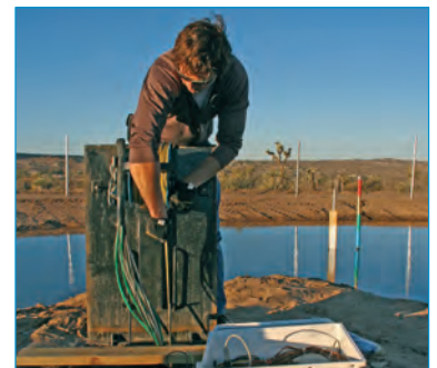
USGS geologist David O'Leary measures the depth to the water table at a pilot-study recharge pond near Yucca Valley.
