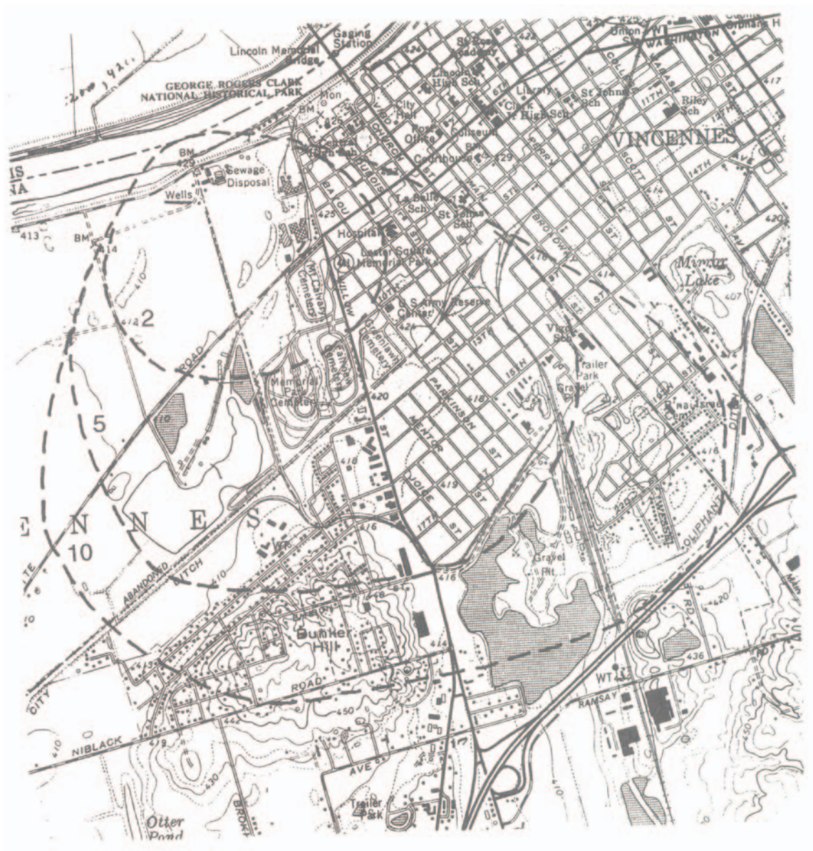
Figure 4.20: Composite time of travel capture zones with 2-,5-, and 10-year isochrones for the city well field using the full-feature analytic element model GFLOW (after [Haitjema,1995]).
