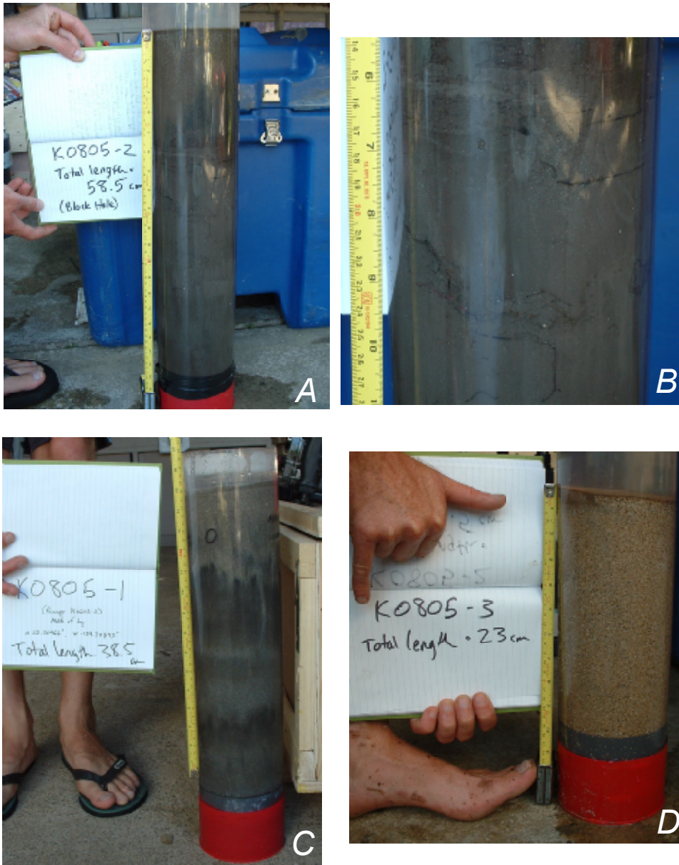
Figure 18. Photographs of sediment cores from Hanalei Bay. A. Mixed mud and sand overlie consolidated mud in sediment from the Black Hole (Core K0805-2, collected in August 2005 from Station F). B. Close-up view of the same core as in A, showing detail of mud with carbonate sand that grades upward into laminated mud containing peat and rare sand. A contact occurs at 15.5 cm, above which laminated mud was present (see appendix 2 for a complete facies description). C. Alternating sandy (lighter) and muddy (darker) horizons in Core K0805-1, collected at Station B in the south-central part of Hanalei Bay. D. Example of the uniform, unconsolidated sand that occurs in many of the cores, with a fine-grained surface 'fluff' layer (Core K0805-3, from Station C on the northeast side of the bay).
