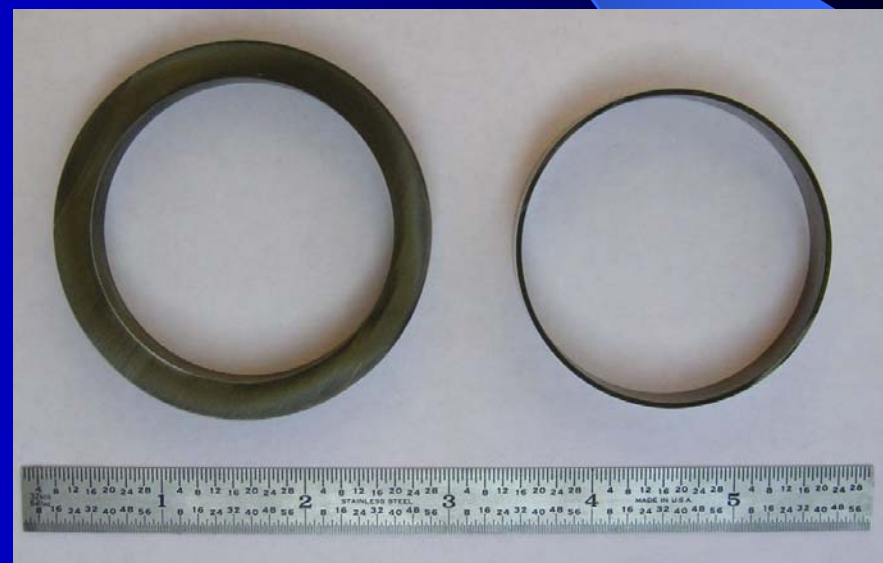
MA956, starting tube 0.25" thick wall. flow formed tube 0.03-0.04"
