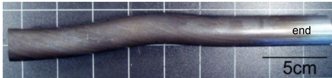
End-section of 2 meter length of PM2000 tube, twisted at Forecr u at 750^{\circ}\text{C} .
