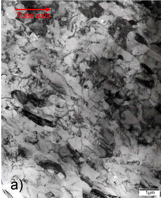
a) torsionally deformed ~20% Plan section. TEM.
