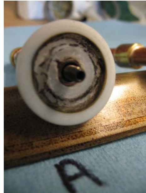
Plasma Burned Microwave Delivery Tube Seal
