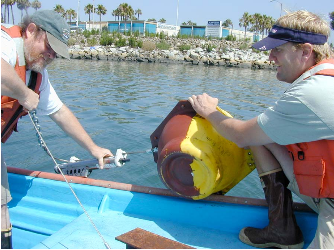
Figure 5. Photo of deployment of surface mooring with Microcat.
