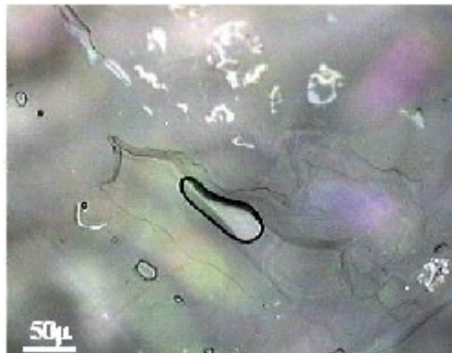
Figure 4. Typical internal blister formation observed perpendicular to the single-crystal \text{Mg}(\text{OH})_2 basal plane surface early during dehydroxylation/dehydroxylation-carbonation reaction processes. As dehydroxylation continues, host-matrix cracking disrupts the blisters as the matrix is fractured down to the nanoscale.
