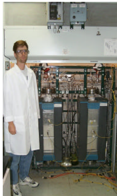
Figure 3. TDA's small-scale fluidized bed apparatus.
