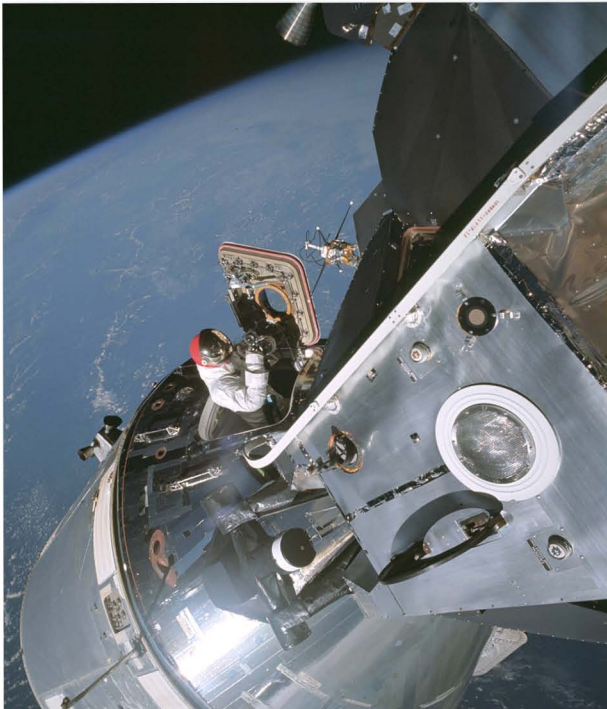
FIGURE 76. —EVA in space. Work in space when an astronaut is outside the protective shell of the spacecraft is always exciting. It is also dangerous and the astronaut must be extra careful. On Apollo 17, the film from the cameras in the SIM must be recovered in this way. Shown here is Astronaut Schweickert during an EVA on Apollo 9. The umbilical hose that connects him to the spacecraft furnishes oxygen and also prevents him from drifting away. Astronaut Dave Scott in the hatch is describing the activities of Schweickert and taking documentary photos. NASA PHOTOS AS9-19-2995 AND AS9-02-3064.
