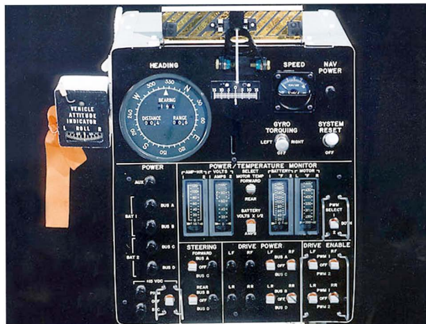
FIGURE 18.—Rover Instrument Panel. This panel contains all of the power switches for the Rover, an indication of the direction in which the Rover is heading, the speed at which it is traveling and the information (direction and distance) necessary to return safely to the LM. Also shown are the power and temperature of various motors. NASA PHOTO S-72-16181.
