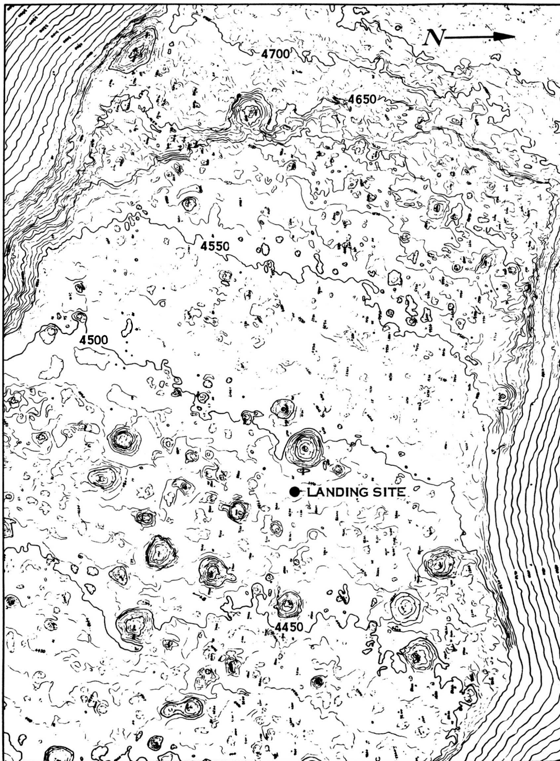
FIGURE 9.—Topographic map of the Taurus-Littrow region. This map shows the elevations of the surface of the Moon in the vicinity of the Apollo 17 landing site. The lines, called contours, connect points of equal elevation. Thus the line that is labeled 4550 indicates that the elevation of all points on the Moon's surface corresponding to that line lies at a relative height of 4550 meters. On topographic maps of the Earth, we measure elevations relative to mean sea level. For the Moon we measure elevations relative to a sphere of radius 1,738,000 meters. The difference in elevation between adjacent lines on the valley floors is 10 meters (about 30 feet); on the steep sides, it is 50 meters. NASA PHOTO 8-72-50327.
