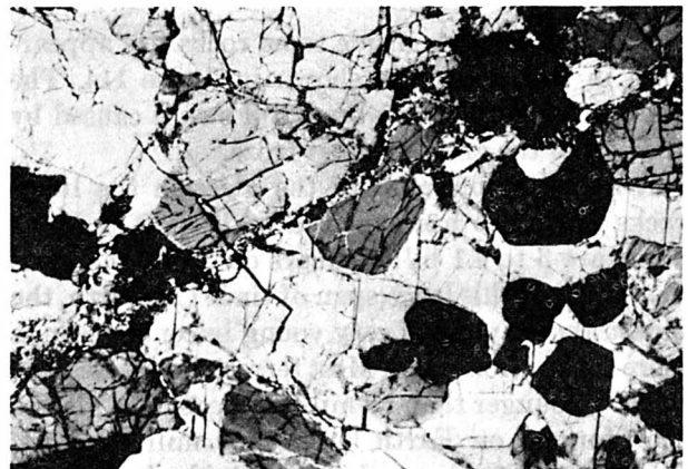
FIGURE 112.—Photomicrograph of Apollo 16 lunar igneous rock 67435. Note distinctness of the individual mineral grains. See text. NASA PHOTO S-72-42390.
