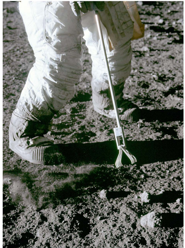
FIGURE 46. —Tongs shown in use on Appollo 12 to collect a small rock. NASA PHOTO S-71-31075.
