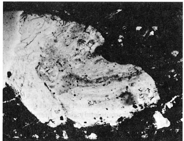
FIGURE 114.—Photomicrograph of lunar rock. This photo taken through a microscope shows the typical appearance of lunar glass. Most of the material in this field of view is glass. Note especially the swirls; they were caused by flow of the glass when it was still fluid. NASA PHOTO 8-71-23092.
