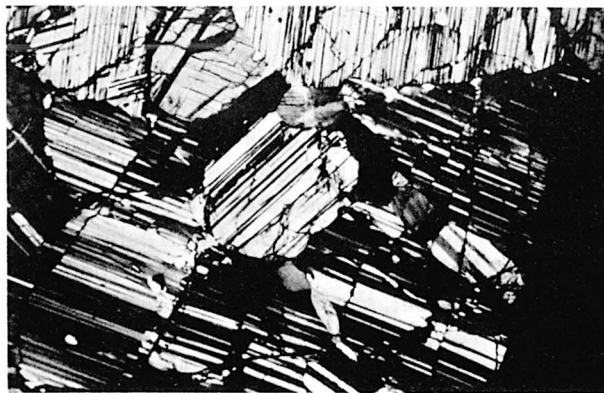
FIGURE 116.—Lunar Anorthosite. This photomicrograph shows that the rock is almost entirely feldspar; therefore, the rock is an anorthosite. Small amounts of other minerals may be seen here as small lightish grains enclosed within grains of feldspar. NASA PHOTO 8-71-51778.
