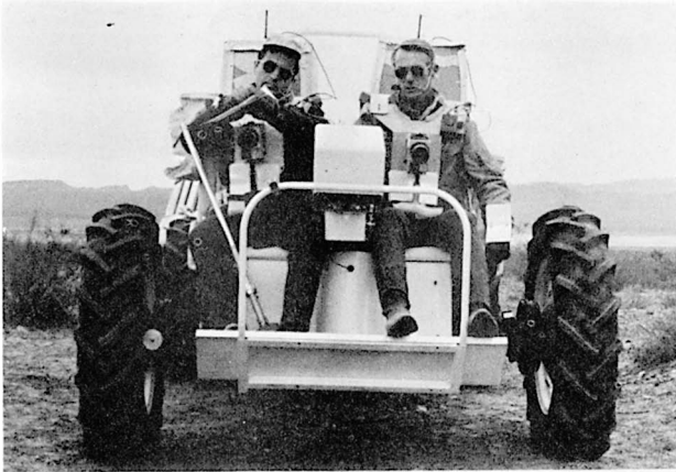
FIGURE 100. —Schmitt and Cernan ride the Explorer. The only model of the lunar Rover used for training is kept at the Kennedy Spacecraft Center. So the U.S. Geological Survey built an inexpensive version, nicknamed Explorer, for use on geological field trips. NASA PHOTO 8-72-30173.
