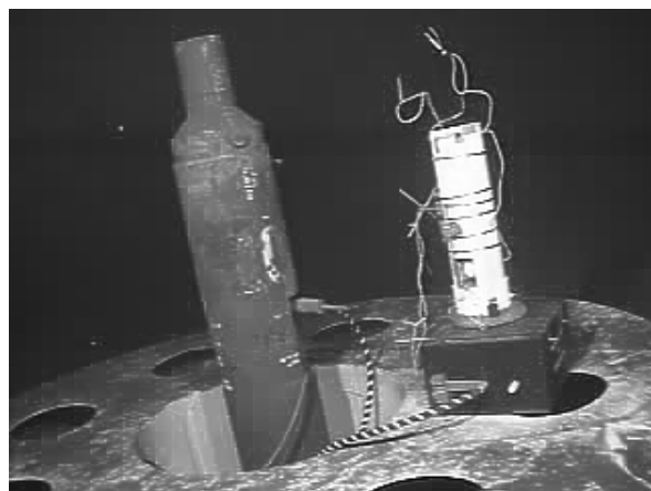
Fig 2.1.6c– Circulation Obviation Retrofit Kit (CORK) structure on top of ODP borehole 1026B. Cylinder and box to right are sampling device “plumbed” into the fluid access port of the CORK.
