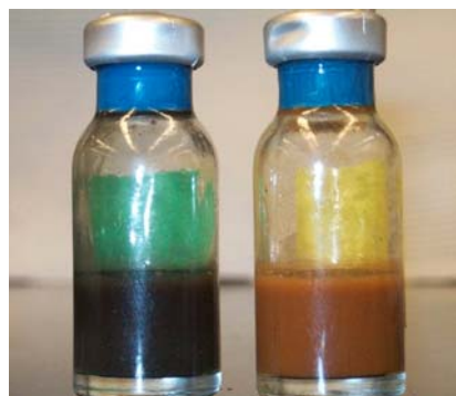
Fig. 17 Fe(III) reduction (upper panel) and reduced Fe mineral production (lower panel) in anaerobically- incubated Fe seep materials with (left) and without (right) electron donor amendment.
