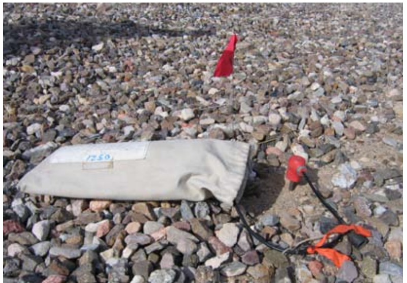
When a series of geophones such as these are placed on the ground, they measure the time it takes a seismic impulse to travel through the soil. This gives experts key information for the Seismic Hazard Analysis.
