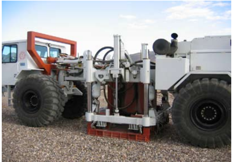
The Liquidator produces vibrations in the ground. Scientists monitor these readings to gather information on the seismic properties of the soil.
