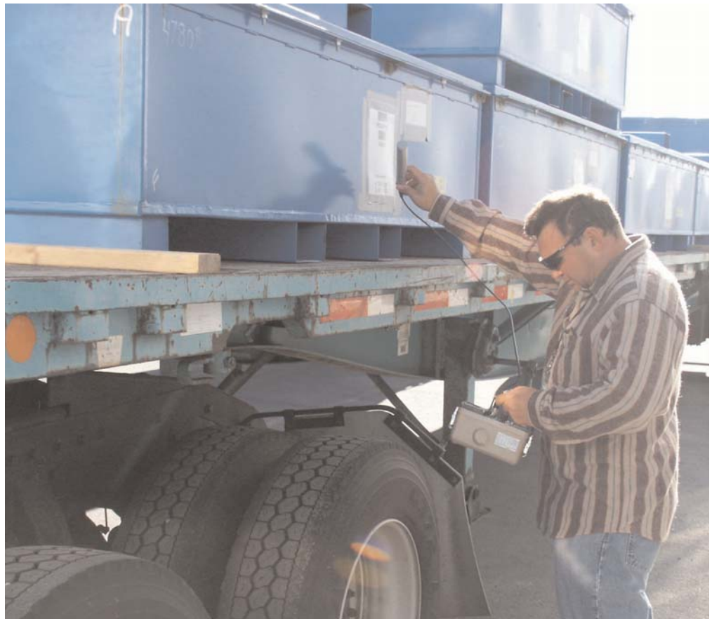
Prior to entering the disposal cells in the Area 5 Radioactive Waste Management Complex, trucks carrying low-level waste are surveyed.
