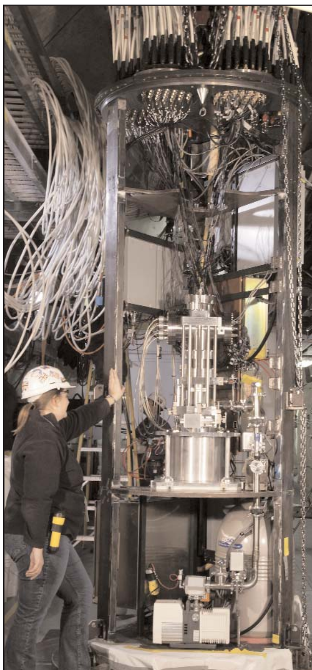
Krakatau subcritical experiment is being prepared to be lowered into the floor of the tunnel of the U1a Complex at the Nevada Test Site.
