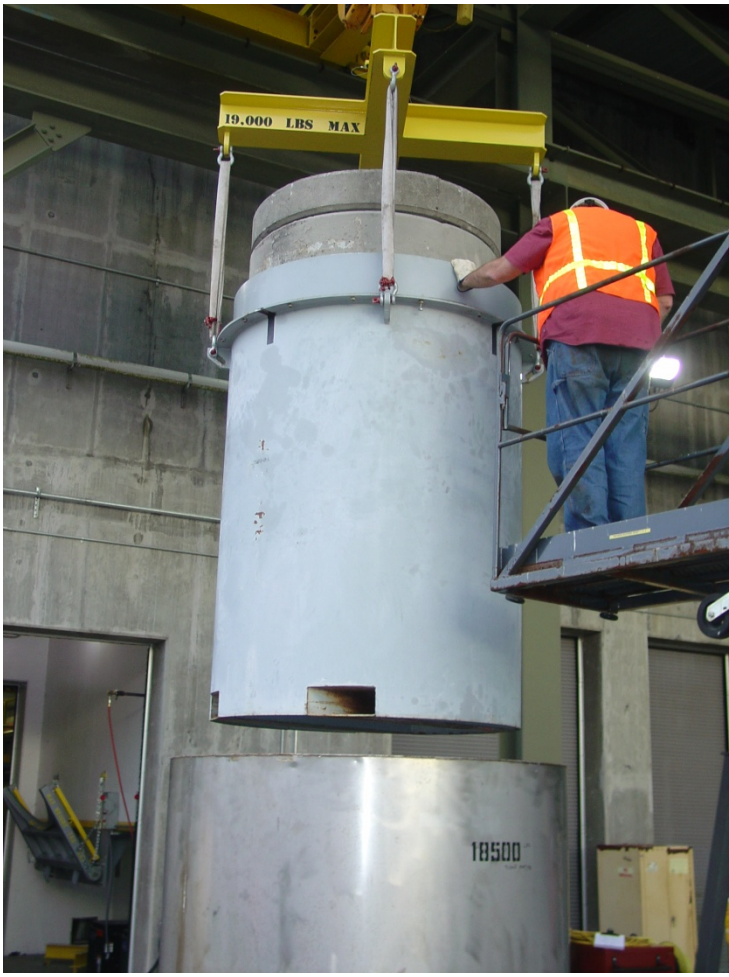
RH Waste Cask Preparation for Insertion Into Hot Cell
