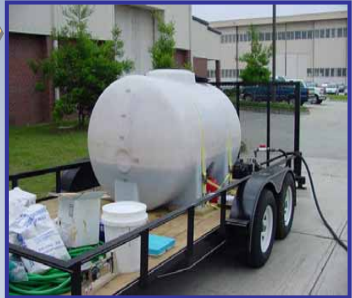
Mobile Batch Injection Trailer
