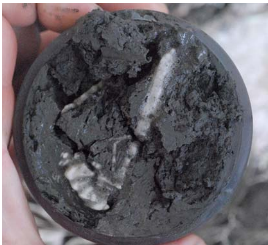
Figure 3| Massive gas hydrate recovered from a core at Site 10. The gas hydrate is white and occurs along a high-angle fracture [4].
