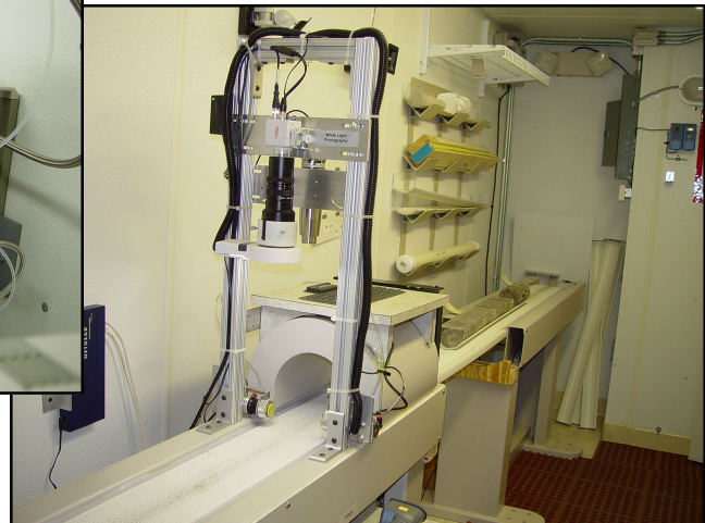
The Mobile Core Lab also includes automated instruments for measuring gamma ray emissions and infrared temperatures.
