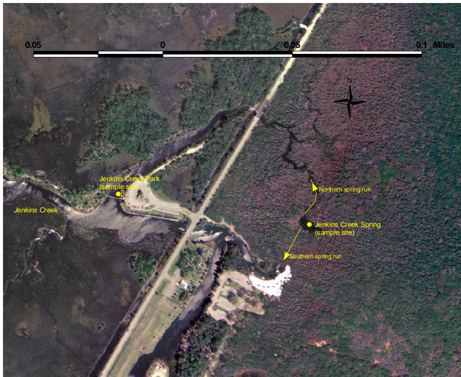
Figure 21. Jenkins Creek Spring with locations of spring runs and sampling sites noted.
