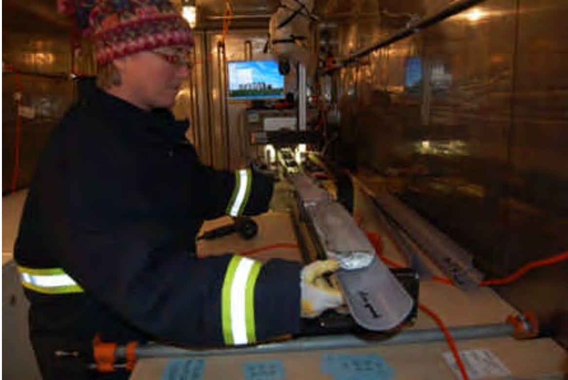
Figure 10, Step 7: Core sections in liner were placed on the Geotek imaging track.
