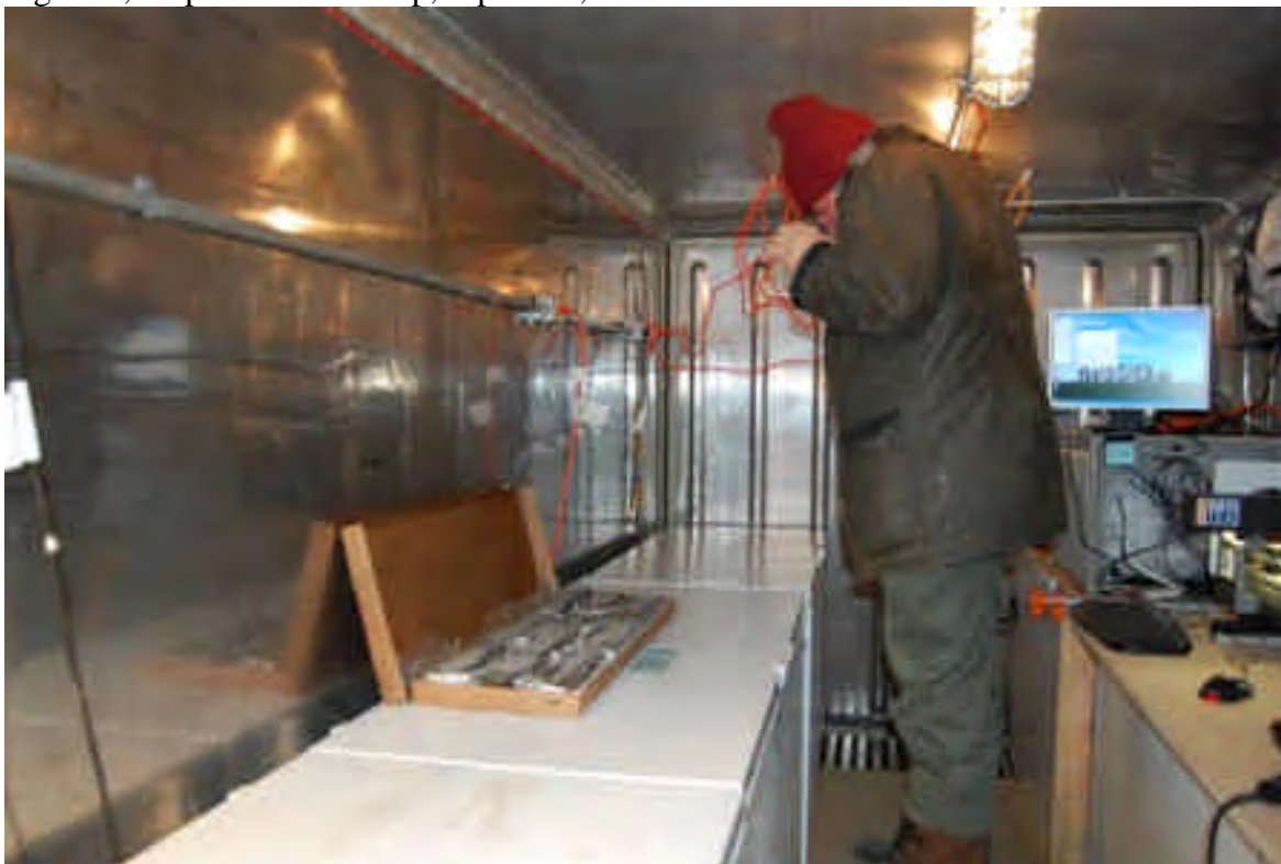
Figure 7, Step 4: The core box including a hand-written label was photographed for records.
