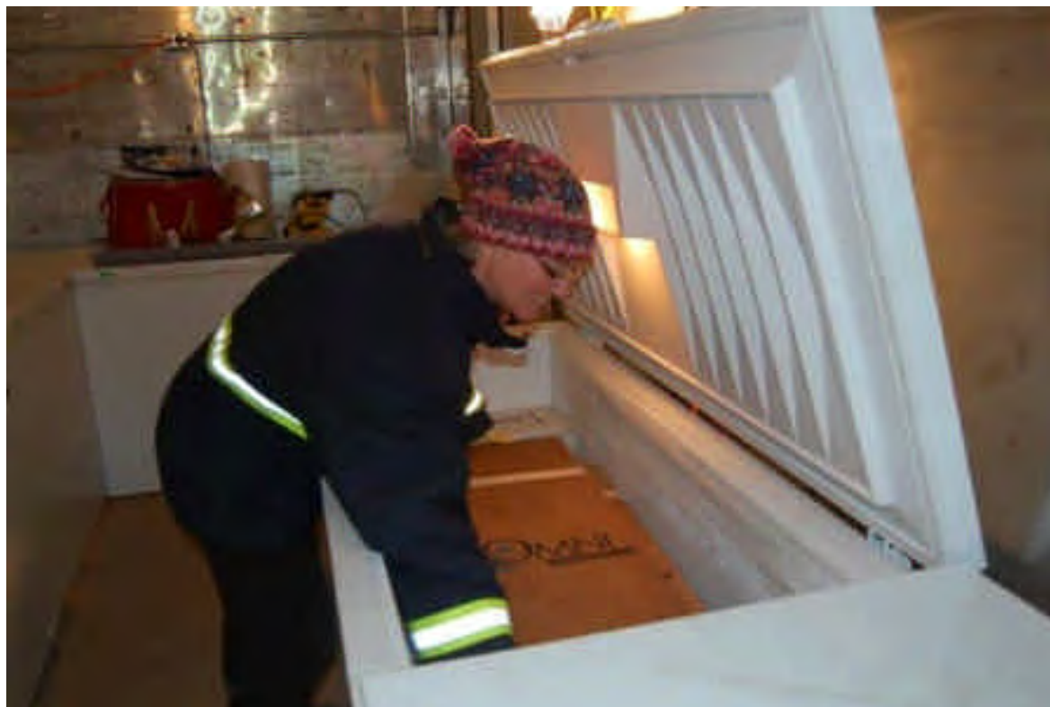
Figure 4, Step 1: Boxes of library set core sections were removed from the freezer (temperature ~20°F), one at a time.
