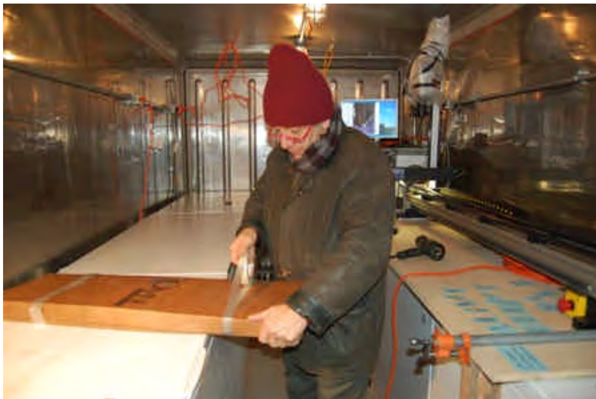
Figure 18, Step 15: Core storage boxes were closed with strapping tape wrapped around each end.
