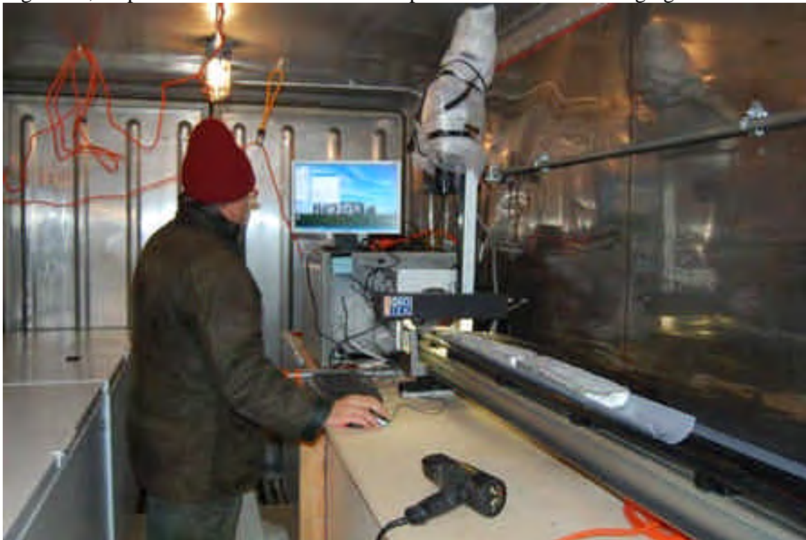
Figure 11, Step 8: Cores were scanned at a resolution of 200 pixels per centimeter at a single set of lighting and aperture conditions, and the camera was consistently calibrated with an 18% grey card so that each image is comparable with every other image.
