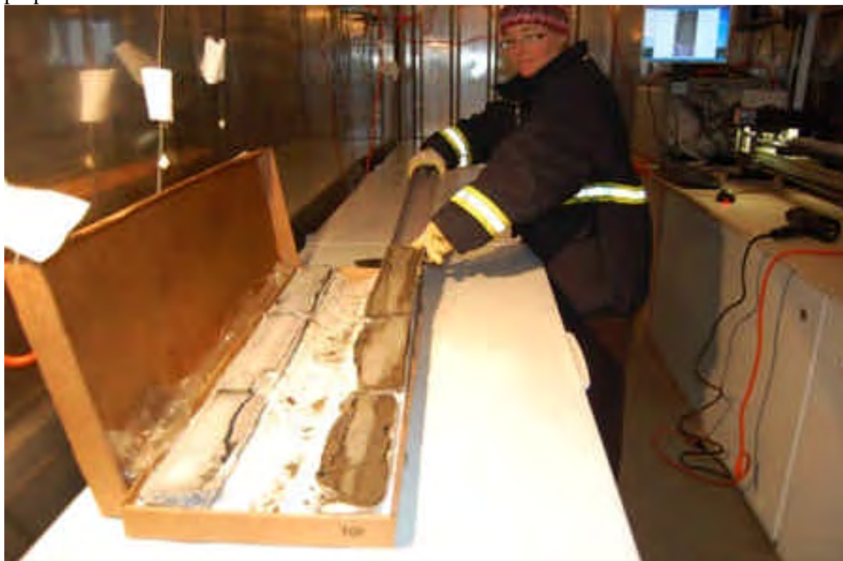
Figure 15, Step 12: The core sections were gently removed from the track in the liner and placed back into the core storage box.
