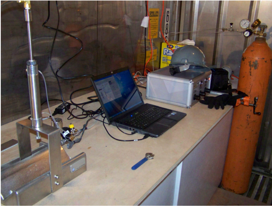
Figure 23: UAF Minipermeameter feasibility test setup in gas hydrate core storage unit (March 2008)
