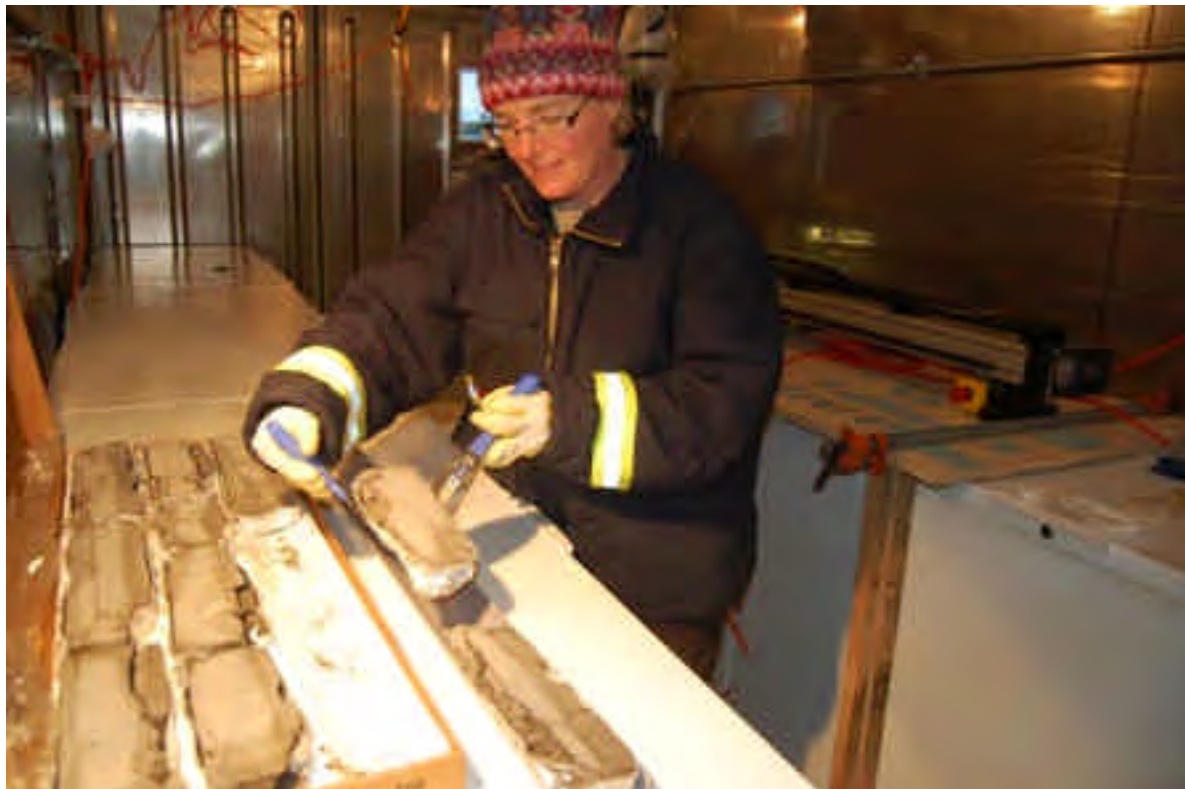
Figure 8, Step 5: Core sections were carefully placed into one-third liners (see "Potential Artifacts," below).
