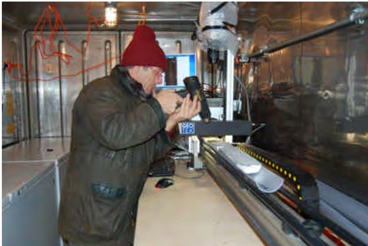
Figure 12, Step 9: Core surfaces were heated using a heat gun to melt surface frost, typically resulting in a wet surface when imaged (see "Potential Artifacts," below).
