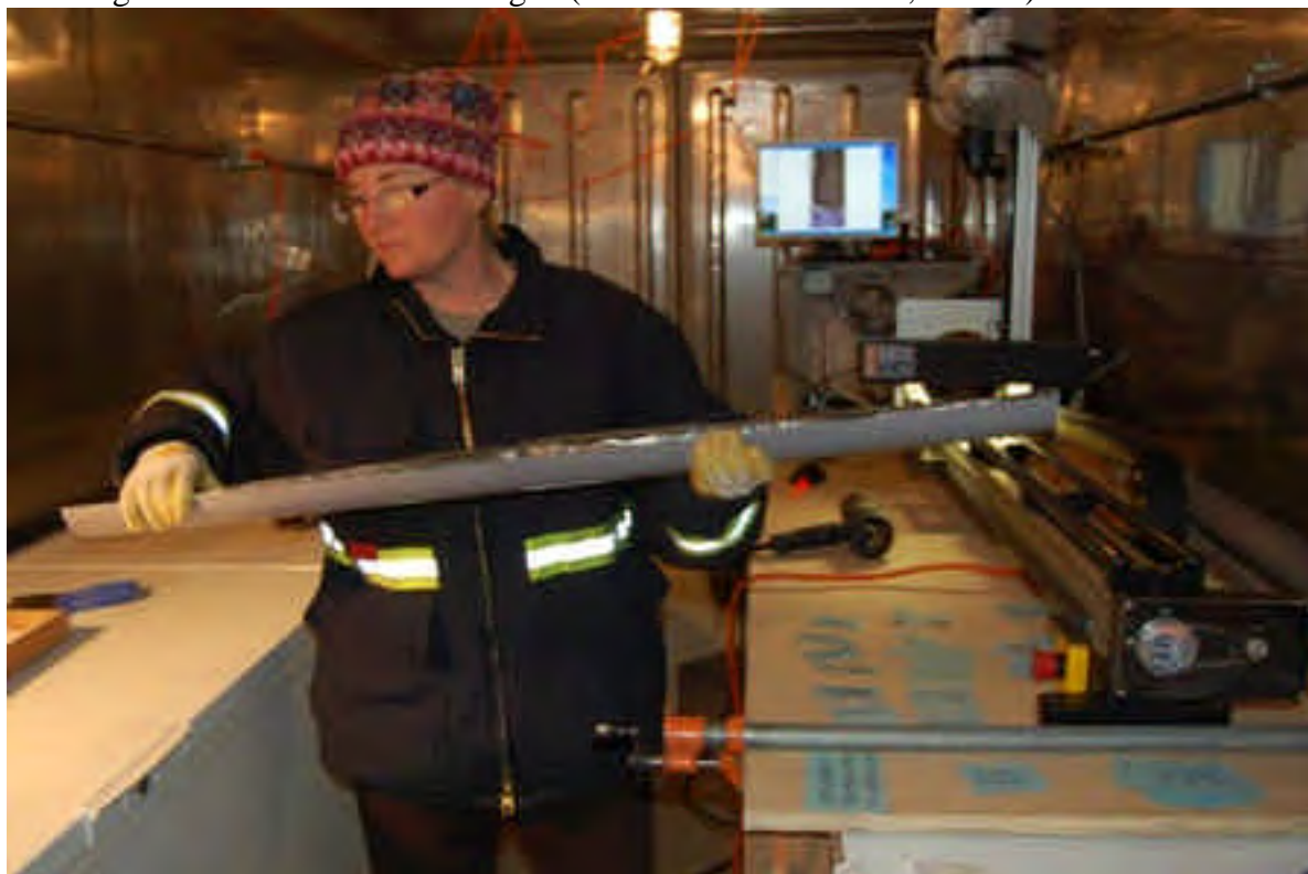
Figure 13, Step 10: Core sections within the liner were removed from the camera track.
