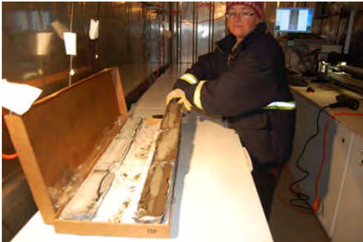
Figure 14, Step 11: The core sections in the core liner were aligned with the core box in preparation for removal.
