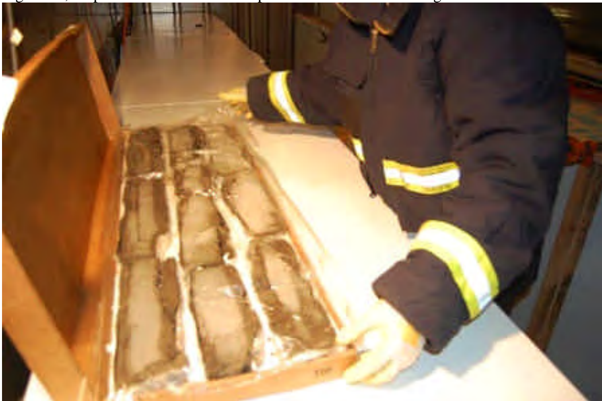
Figure 17, Step 14: Plastic wrap, if present, was replaced over the core surfaces. Bubble wrap (flat side to the core) was substituted if no plastic wrap was present.
