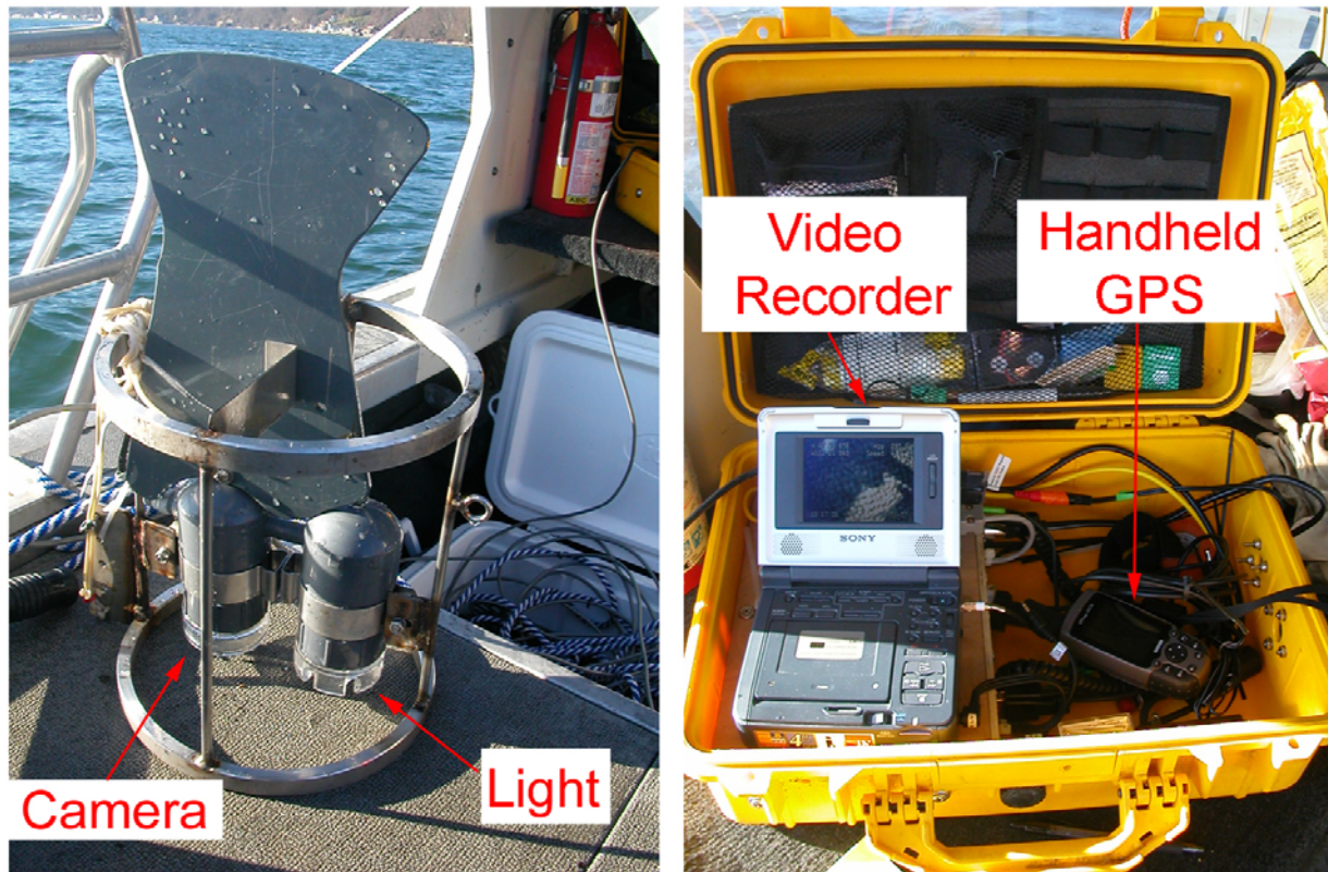
Figure 4. Photographs showing the main components of the underwater video system.
