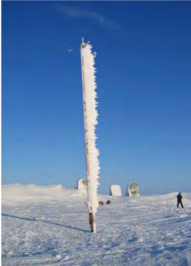
Figure 5.10. Nome Anvil Mountain, Met-Tower after icing event.
