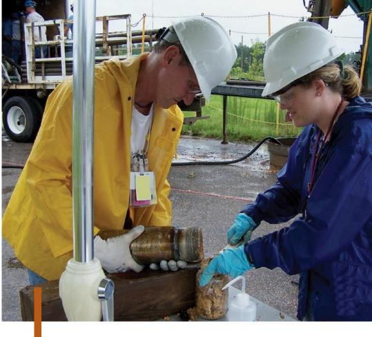
National laboratory scientists prepare soil samples to study how well the subsurface can naturally attenuate contaminated groundwater.
