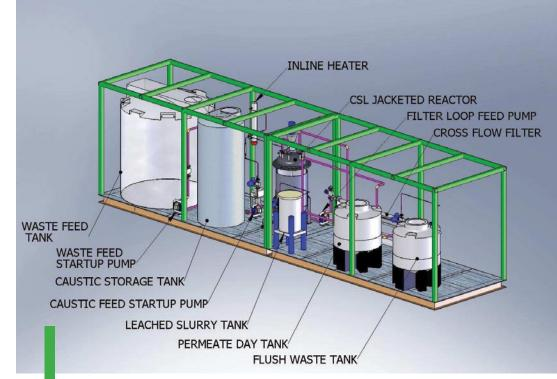
Continuous Sludge Leaching is being tested as an option to remove aluminum from tank waste to reduce the volume of waste feed to the Hanford Waste Treatment and Immobilization Plant.
