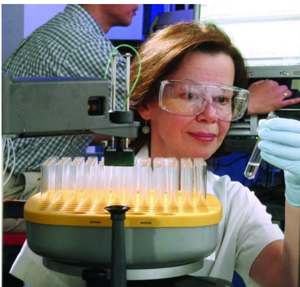
Biochemist and biophysicist at the Midwest Structural Genomics Center work with a robot to automate the protein crystallography process.
