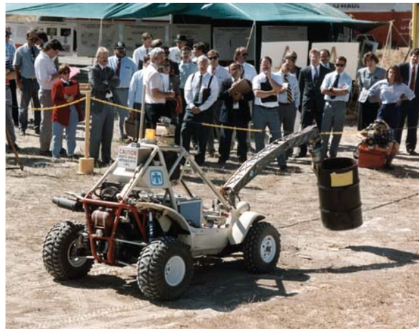
RETRVIR is a Honda all-terrain vehicle equipped with a six-foot robotic arm for digging and picking up pieces of contaminated material and placing them in storage containers. RETRVIR drives itself using automatic planning software.
