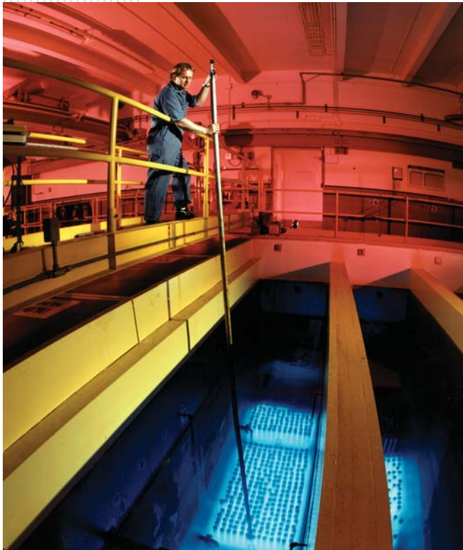
The Hanford worker shown here in the Waste Encapsulation Storage Facility is using a pole manipulator to pick up cesium capsules under water to move them to another location in the pool and/or test them by a rapid up and down movement to verify that the inner capsule still moves. This is known as the "clunk test."
