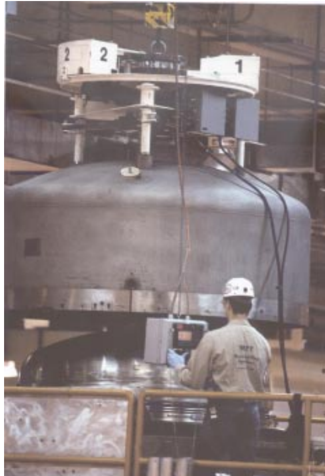
Removing outer lid at the Waste Isolation Pilot Plant
