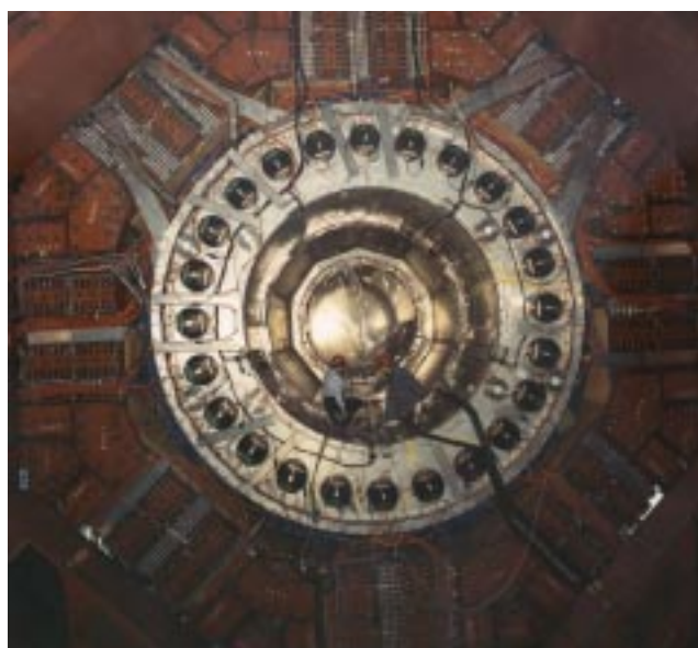
The Stanford Linear Accelerator Center is a national basic research laboratory, probing elementary particle physics and developing new technology in high energy accelerators and elementary particle detectors. Photo depicts a cross-section of the large detector where electrons and positrons collide.
