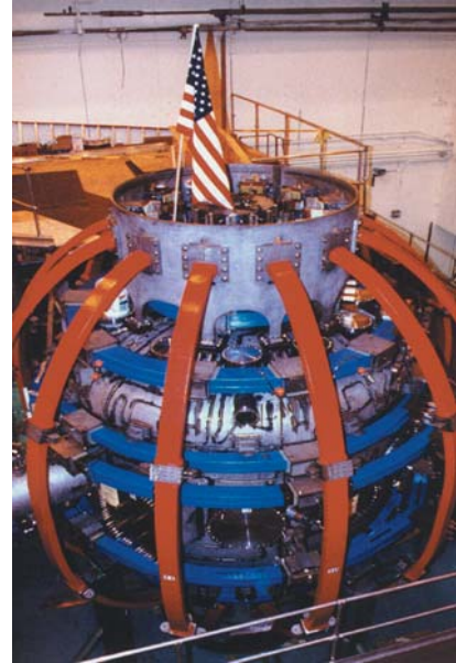
National Spherical Torus Experiment (NSTX), a magnetic fusion device constructed by Princeton Plasma Physics Laboratory (PPPL) in collaboration with Oak Ridge National Laboratory (ORNL), Columbia University, and the University of Washington, obtained first plasma on February 12, National Spherical Torus Experiment 1999. NSTX will be used to study physics principles of spherically shaped plasmas—hot ionized gases in which nuclear fusion will occur under the right conditions of temperature, density and confinement in a magnetic field.
