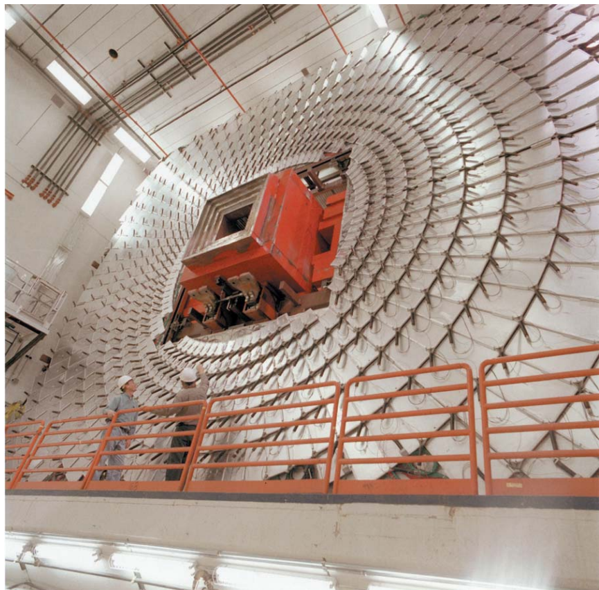
FERMI'S two detectors, the collider detector facility (CF) and the D-Zero, are about four stories high, and weigh about 5,000 tons each. The particle collisions occur in the middle of the detectors, which are crammed with electronic instrumentation.
