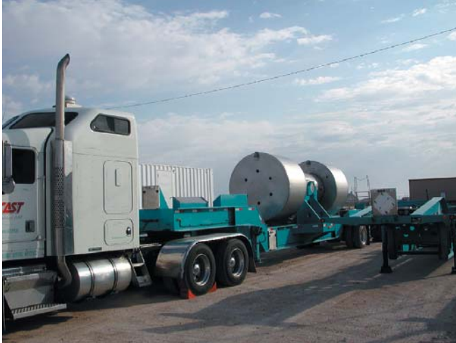
Picture of the first NRC certified RH-72B cask at the Waste Isolation Pilot Plant (WIPP) at Carlsbad, NM. This type of cask will be used to transport remote-handled transuranic waste from DOE sites around the country to WIPP for disposal.
