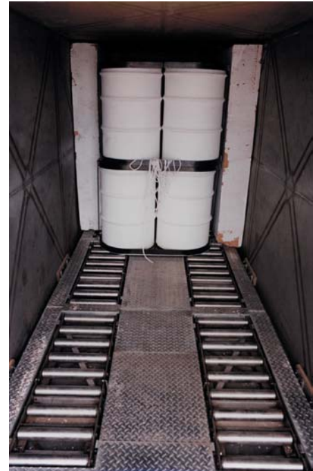
View of two “six-packs” within transuranic package transporter’s (Trupact) storage compartment. The trupact was designed to safely ship defense nuclear waste materials to storage sites and repositories.
