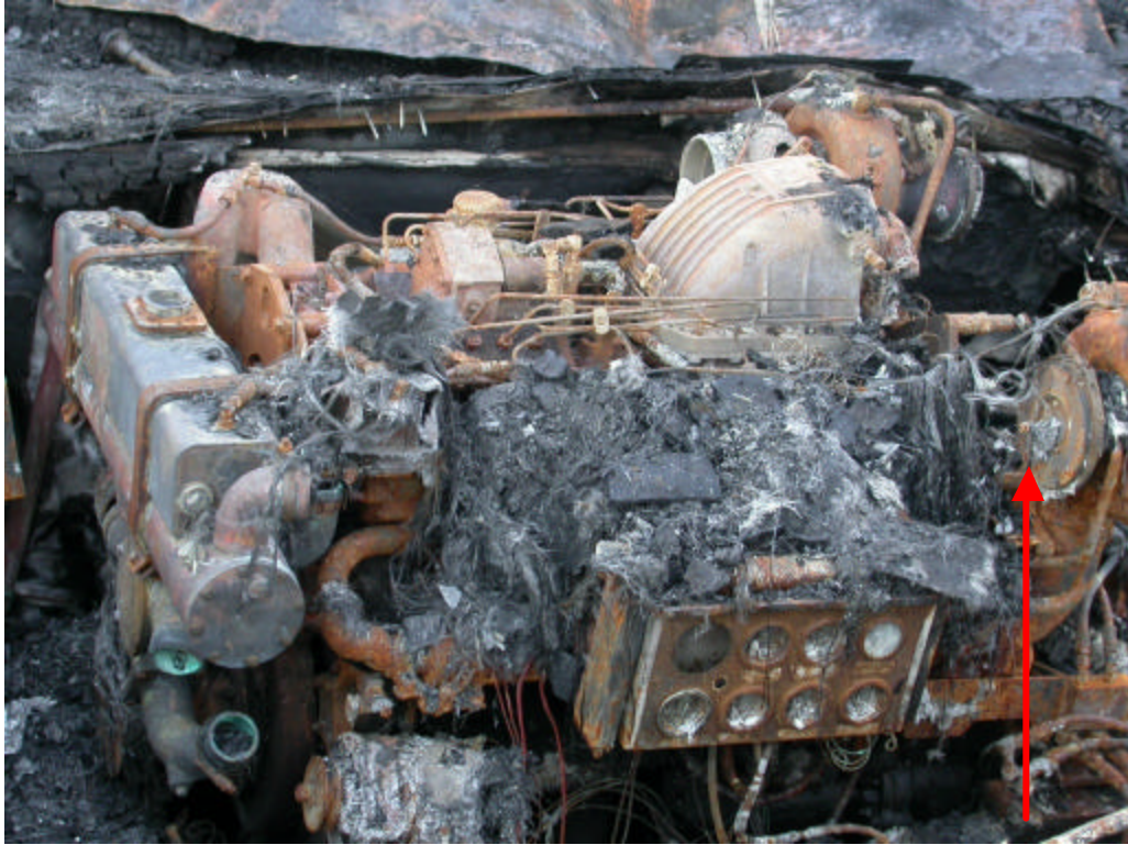
Remaining Turbocharger Impeller
